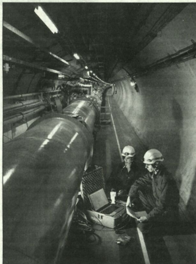
"Engineers checking the electronics on a LHC dipole magnet. (Image by: Maximilien Brice; Claudia Marcelloni copyright CERN)"
