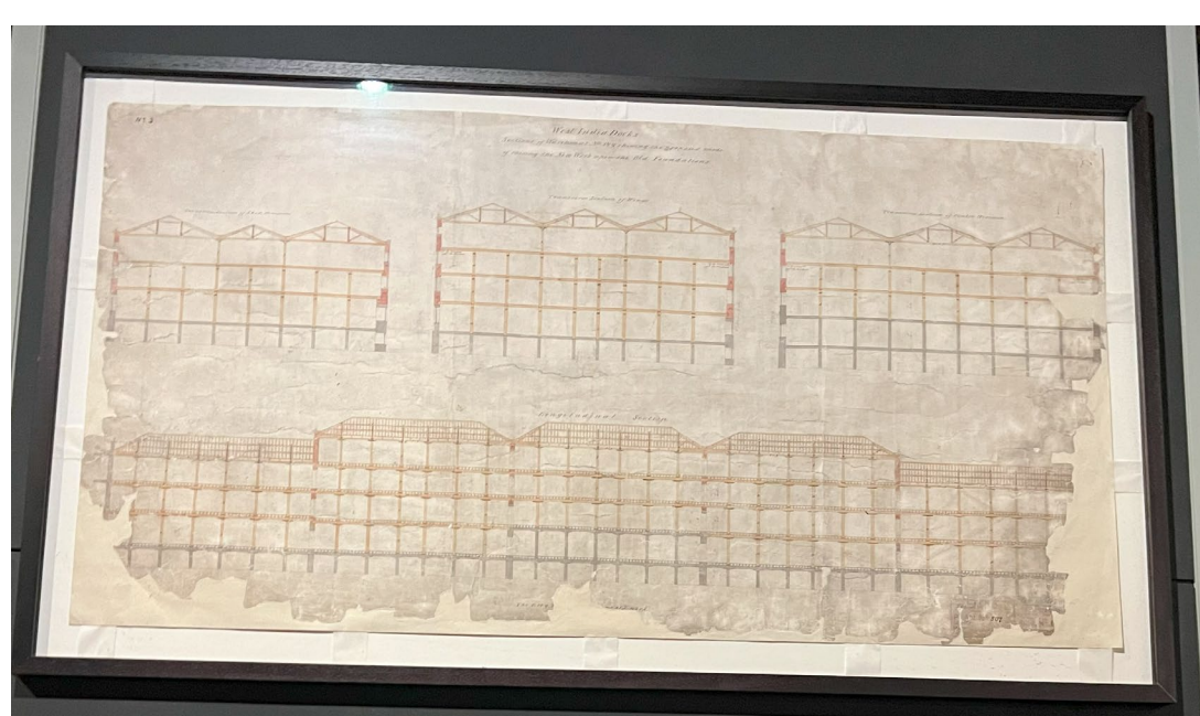
Internal Sections of Nos 1 and 9 Warehouses: This helps us to examine what the building looked like before renovation when it was still a sugar mill in 1827.
