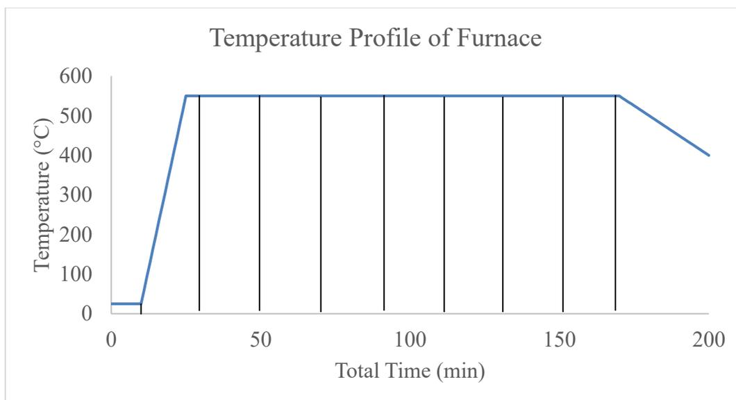
Figure 3. Temperature Profile of Furnace. Vertical black lines represent times when TCD measurements were taken.
