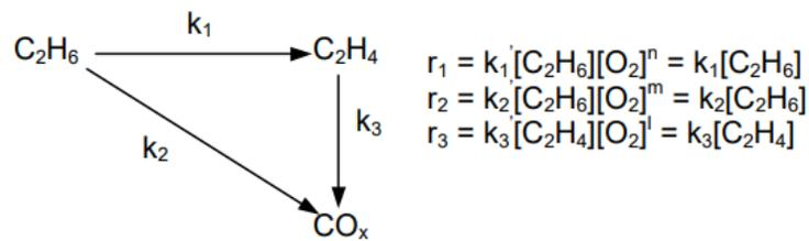
Figure 1. Reaction pathways for ethane ODH.
