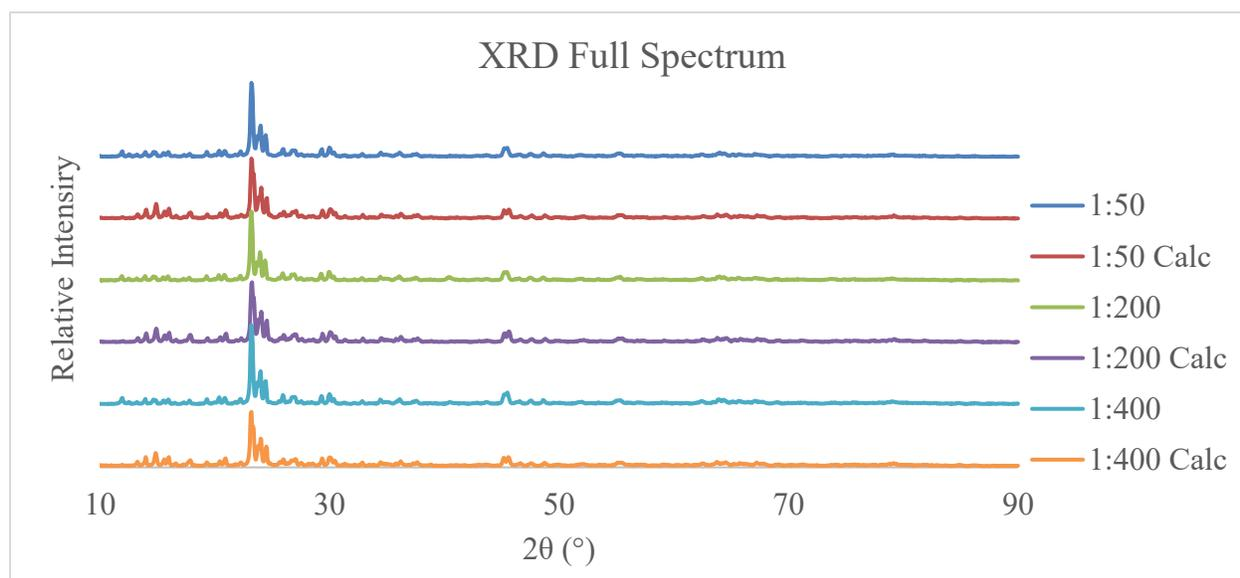
Figure 4. The XRD peaks are shown for uncalcined and calcined samples of Fe:Si ratio 1:50, 1:200, and 1:400.
