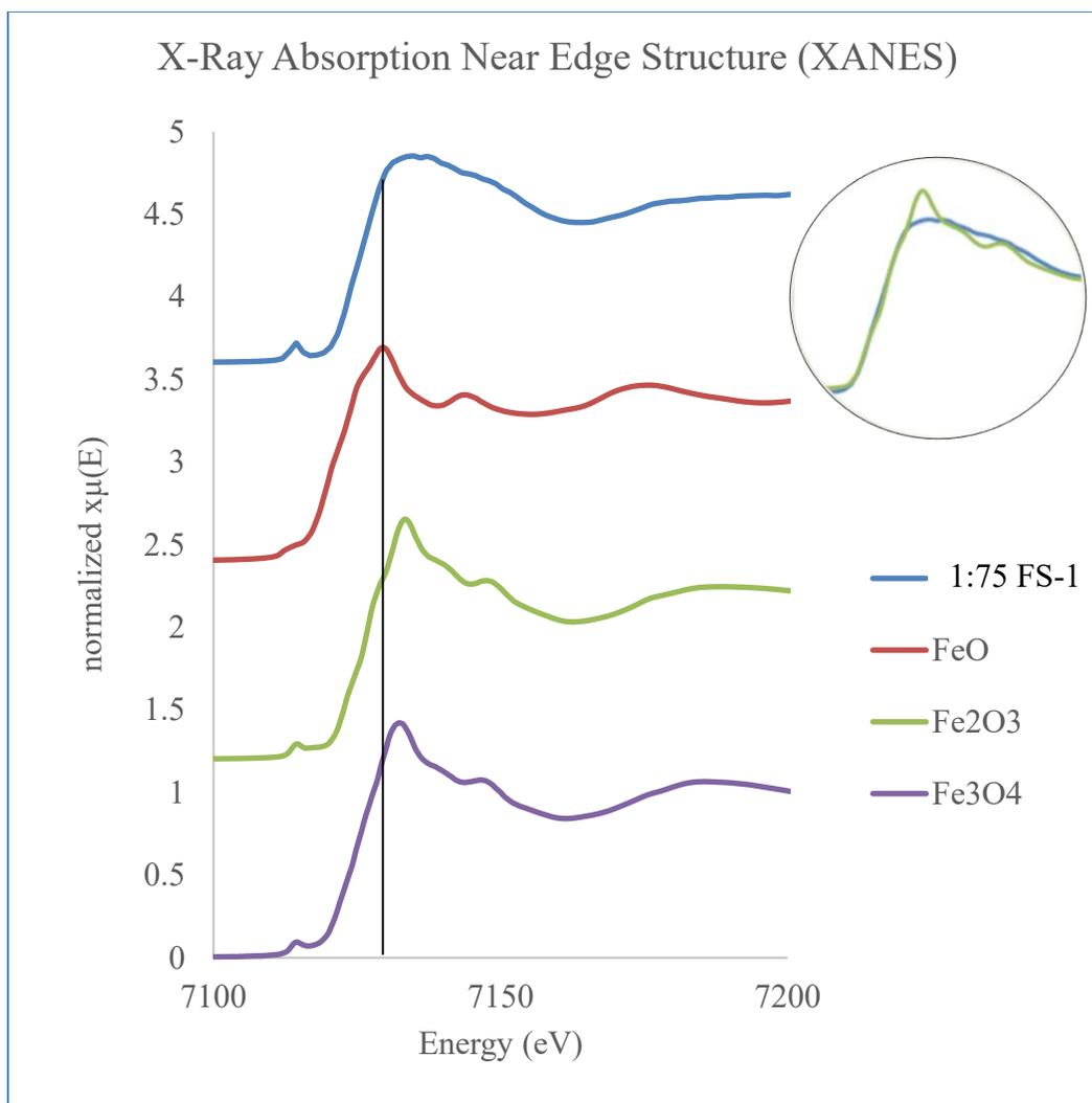
Figure 7. XANES plot comparing 1:75 FS-1 to FeO, Fe<sub>2</sub>O<sub>3</sub>, and Fe<sub>3</sub>O<sub>4</sub>
