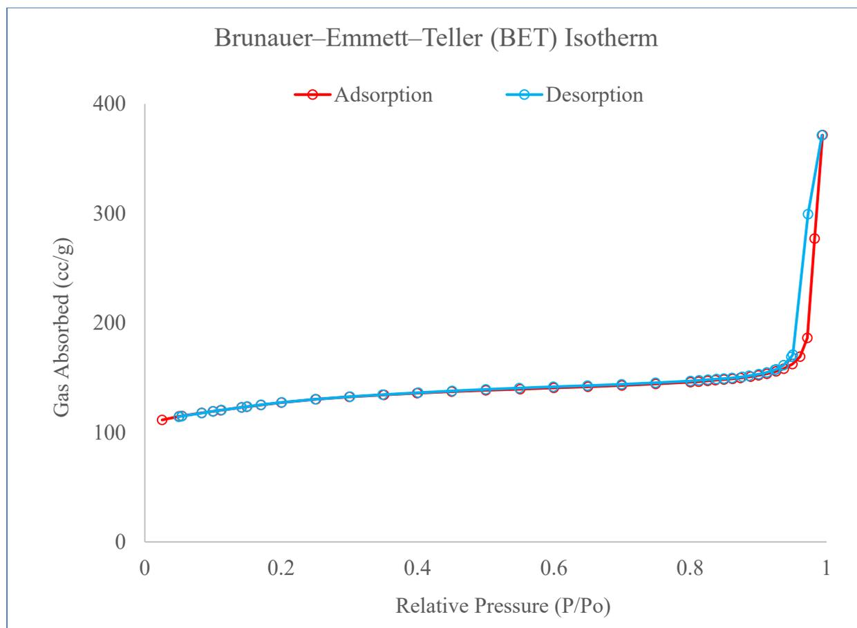
Figure 6. 38 adsorption measurements and 37 desorption measurements were taken using nitrogen at 77 K to obtain the BET isotherm curve.
