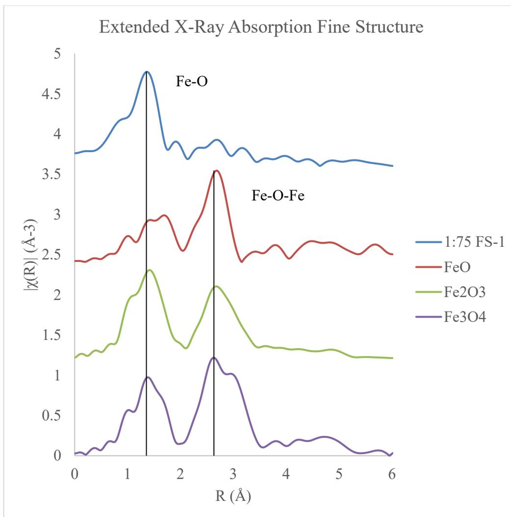
Figure 8. EXAFS plot comparing 1:75 FS-1 to FeO, Fe<sub>2</sub>O<sub>3</sub>, and Fe<sub>3</sub>O<sub>4</sub>
