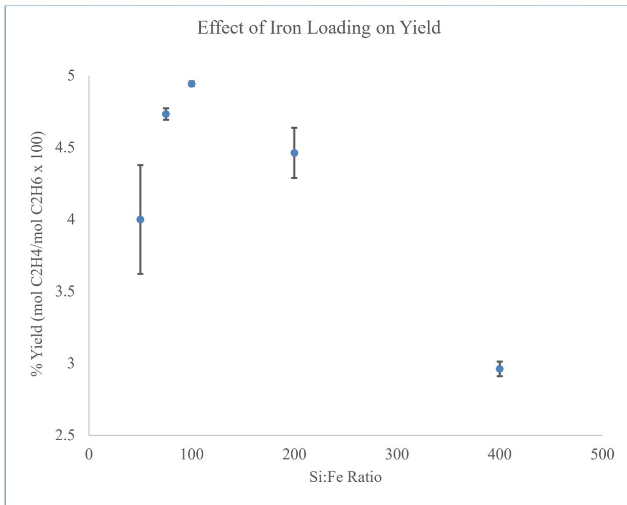
Figure 11. Yield of each of the five samples is plotted with error bars of  $\pm$  one standard deviation.
