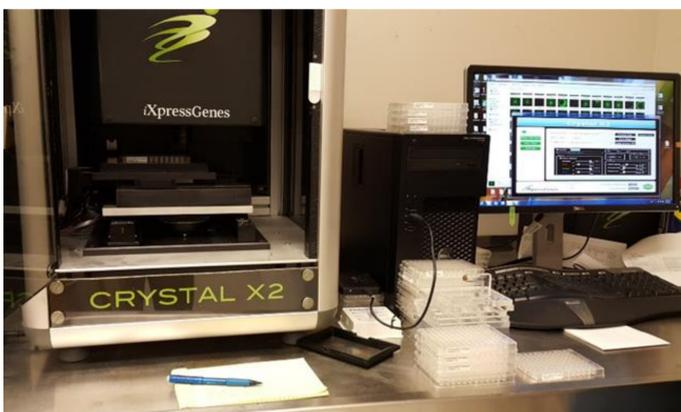
Fluorescent microscope system, Crystal X2, for finding protein crystal leads.
