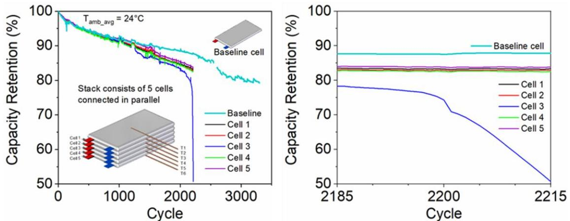
**Figure 1.** Capacity retention of Baseline cell and individual cells in the stack during cycling in our previous studies.
