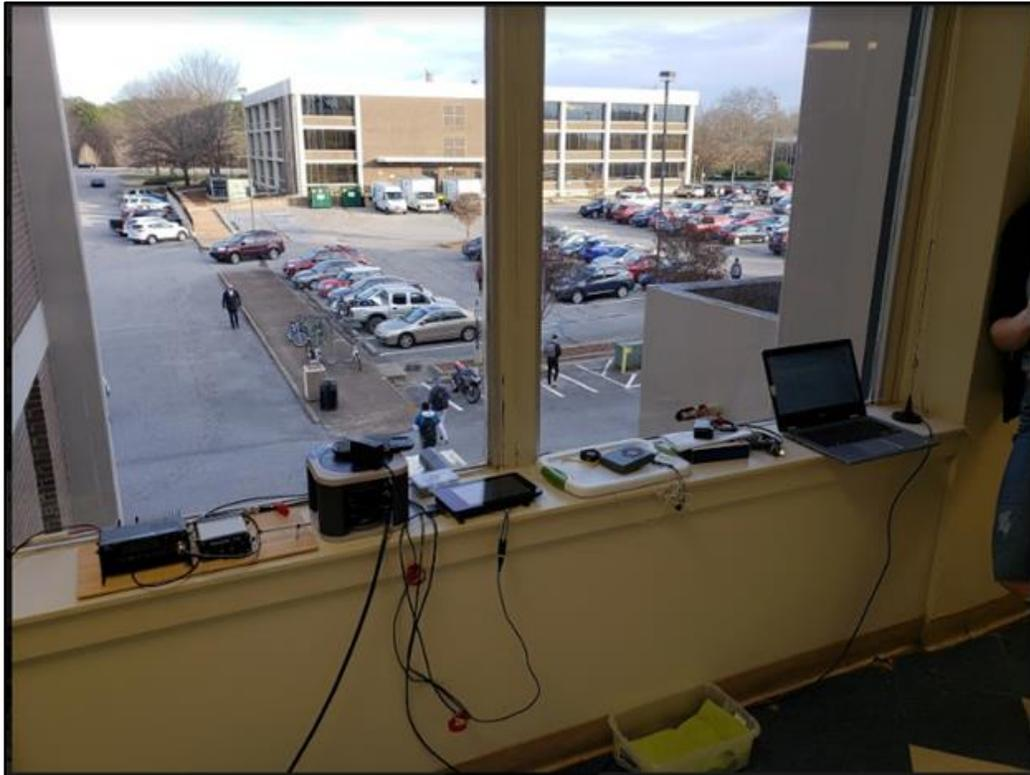
**Figure 1: Raspberry Pi setup, with the microcontroller, radio transmitter and receiver**
