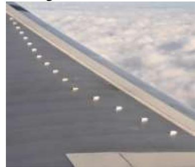
Fig.1: Vortex generators: Preventing stall at high and low speeds. The figure is taken from flickr.
