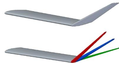
Fig. 1: Top: Single winglet. Bottom: Multi-Winglet – Isometric View.
