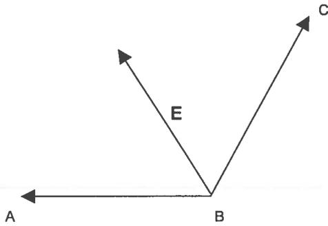
*Diag 1: Computing electric field vector  $\mathbf{E}$ . The Weimer model yields potentials at points A, B, and C; the vector sum is used to obtain the gradient vector  $\mathbf{E}$ .*
