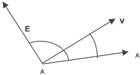
*Diag 2: Verifying orthogonality. The satellite moves from point A to point A'. The angle between the satellite path and the convection velocity is known; that between the path and the electric field vector  $\mathbf{E}$  can be calculated.*
