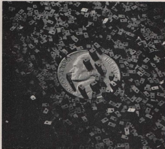
MINUTENESS OF BIAX is shown in this photo of several hundred of the new computer elements with a nickel. More than 5,000 can be held in the palm of your hand, and 310,000 will fit in a quart milk carton. BIAX is now in mass production, and complete BIAX memory systems and computers are now being marketed for special commercial and military applications.
