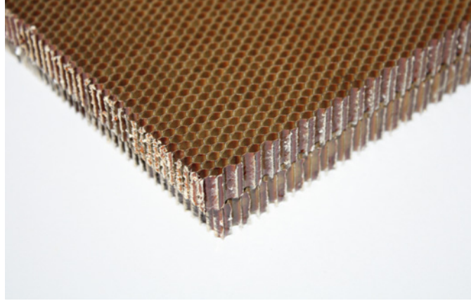
Figure 2.3: Two honeycomb cores offset from one another
