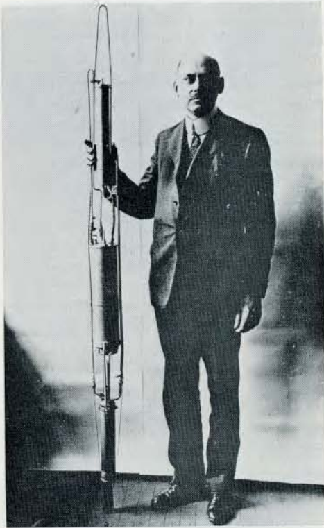
Dr. Goddard in his laboratory at Clark University with the rocket tested on May 4, 1926. This rocket is the second model of a liquid-propellant rocket first flown on March 16, 1926.
