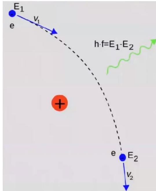
Figure 2: How Bremsstrahlung X-rays are formed
