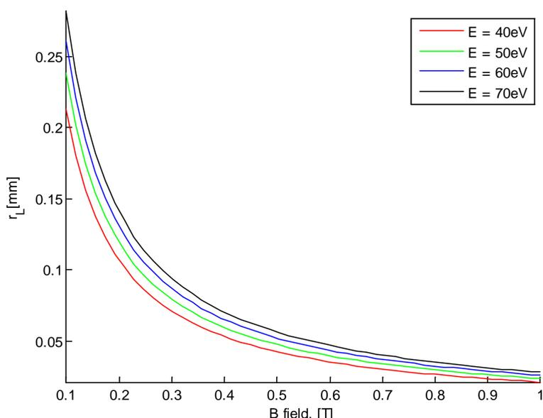
Figure 1: Larmor radius of electrons in a constant B field.
