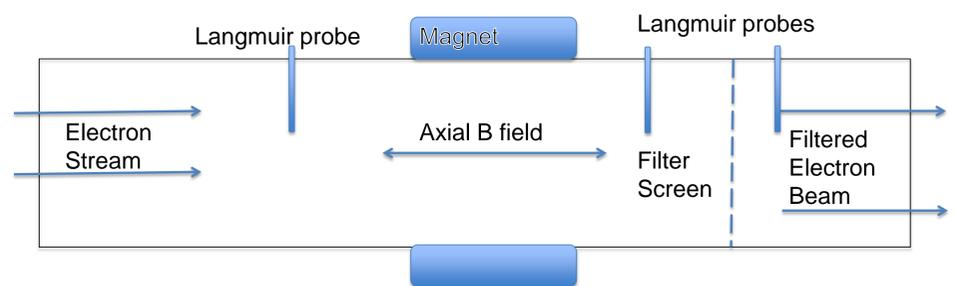
Figure 2: Layout for Electron Beam Filtering Test System
