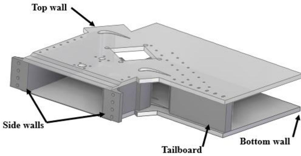
Figure 8: Linear cascade components.
