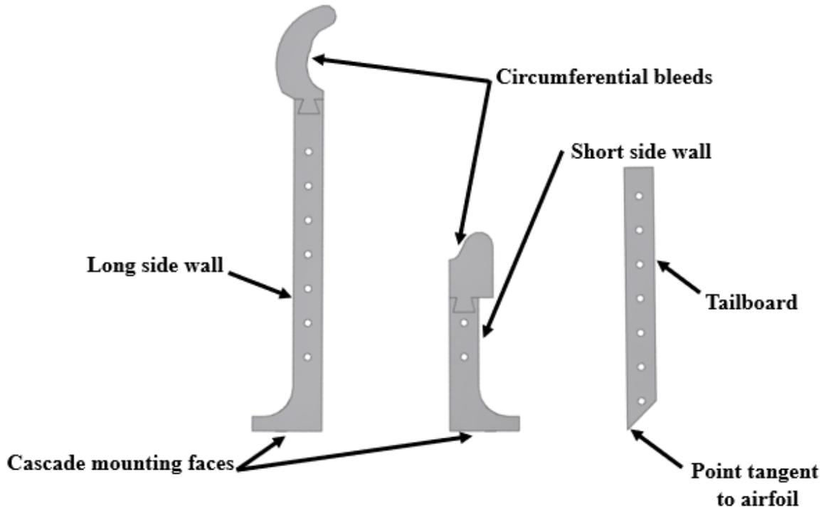
Figure 11: Top view of side wall and tailboard components.
