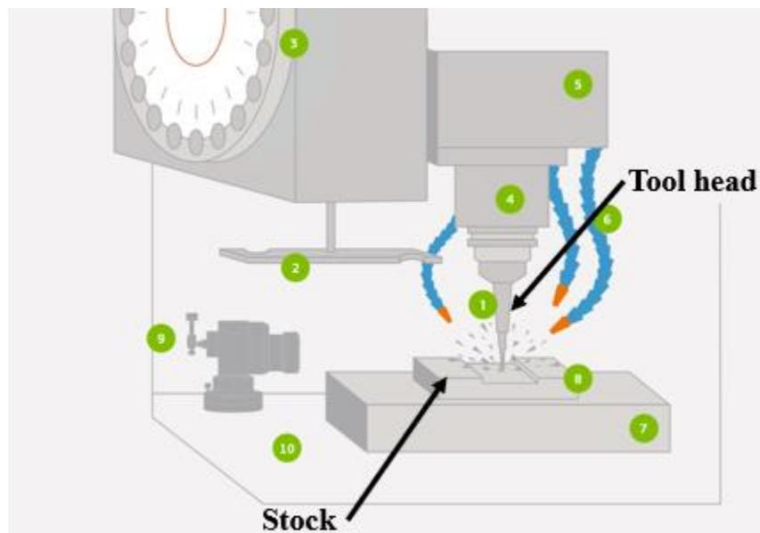
Figure 17: Computer Numerical Control (CNC) machine operation [2].
