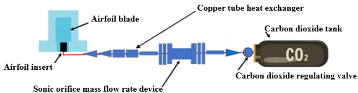
Figure 15: Carbon dioxide supply system components.
