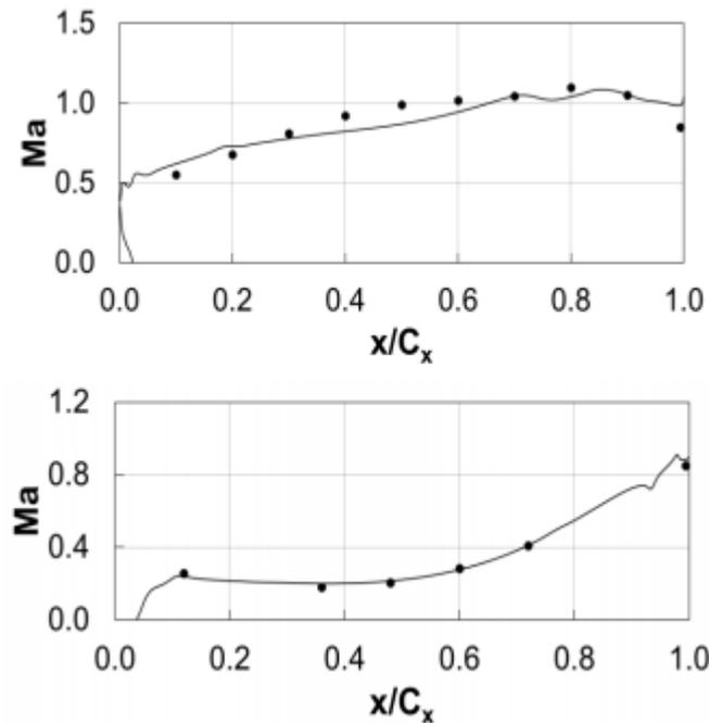
**Figure 19: Mach number distributions on the suction and pressure sides of a baseline turbine blade, as measured at fifty percent span. Solid lines represent predicted data.**
