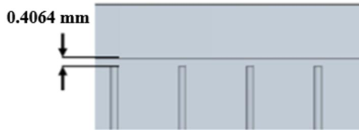
**Figure 7: Thermocouple junction to squealer recess surface distance.**
