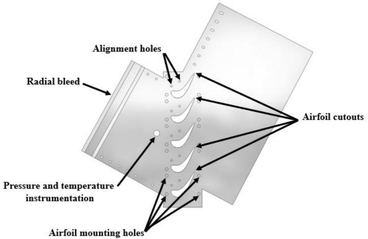
Figure 10: Bottom view of linear cascade bottom wall design.
