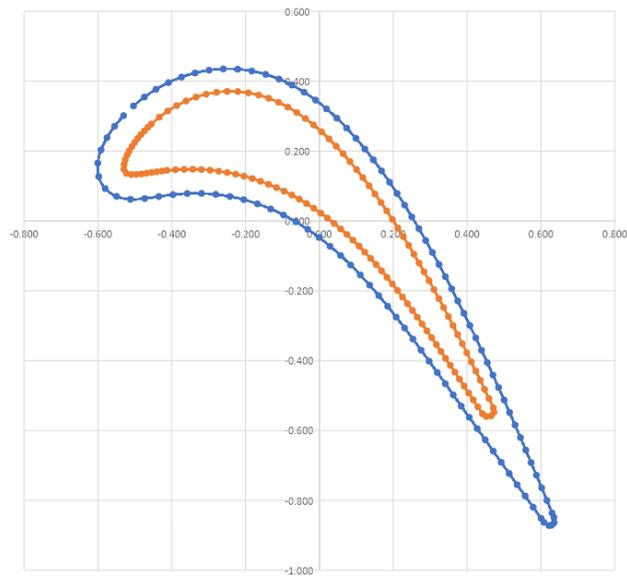
**Figure 1: Turbine blade profile, including squealer recess region.**
