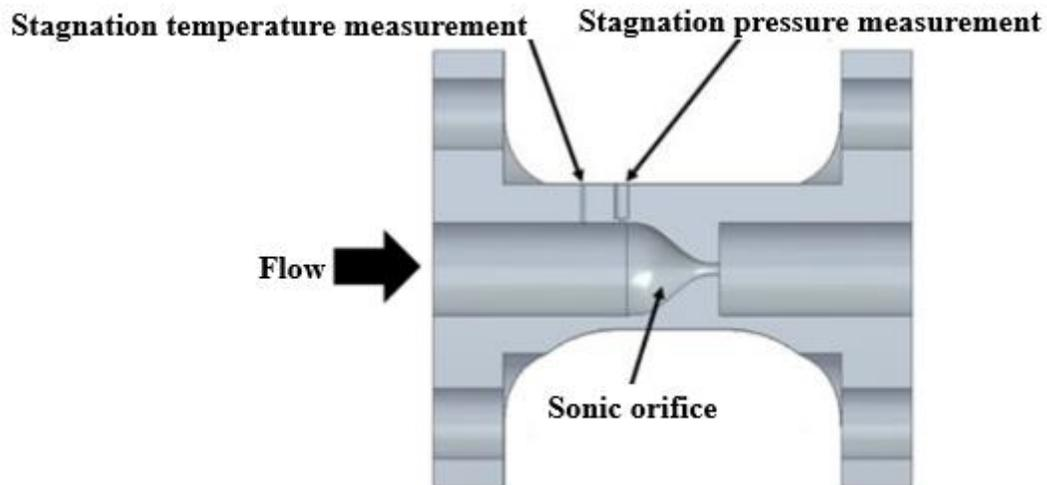
**Figure 14: Sonic orifice mass flow measurement device cross-section.**
