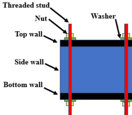
Figure 12: Clamping force assembly for linear cascade top and bottom walls.
