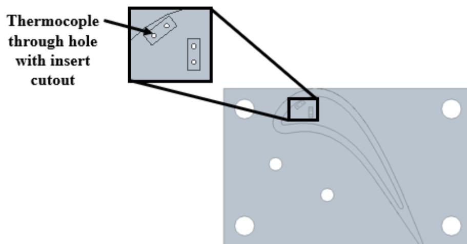
**Figure 6: Surface thermocouple installation tabs as positioned on the blade tip.**
