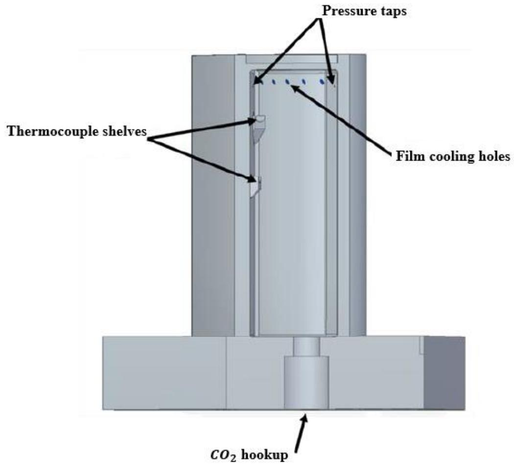
**Figure 4: Cross-sectional view of blade plenum, including instrumentation and the carbon dioxide connection location.**
