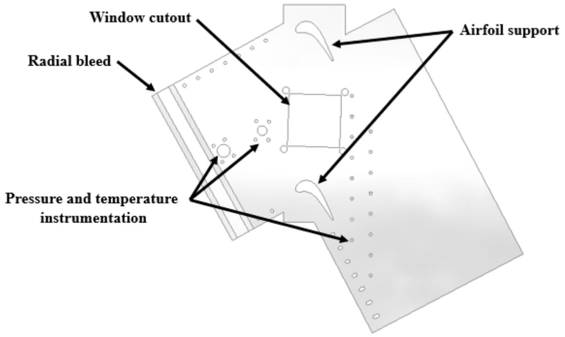
Figure 9: Top view of linear cascade top wall design.
