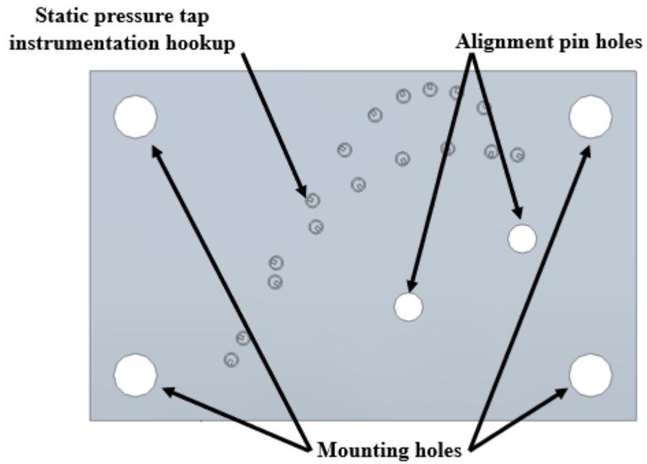
**Figure 3: Bottom view of blade base with static pressure tap locations.**
