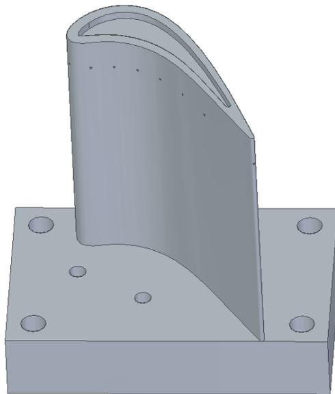
**Figure 2: Turbine blade with squealer and surface static pressure taps located at 90 percent span.**
