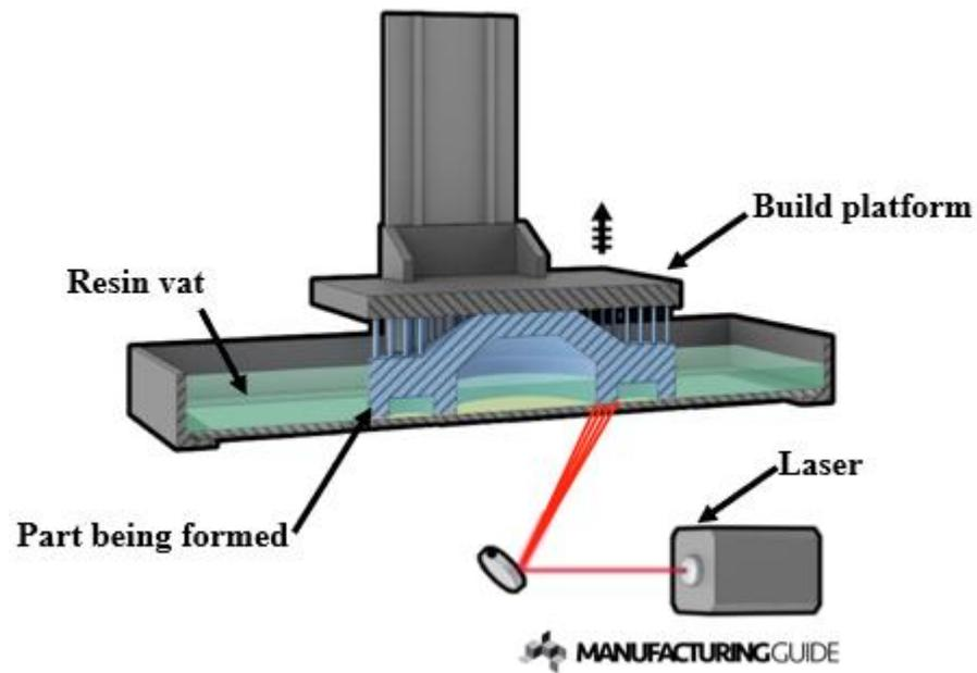
Figure 16: StereoLithography Apparatus (SLA) process [4].
