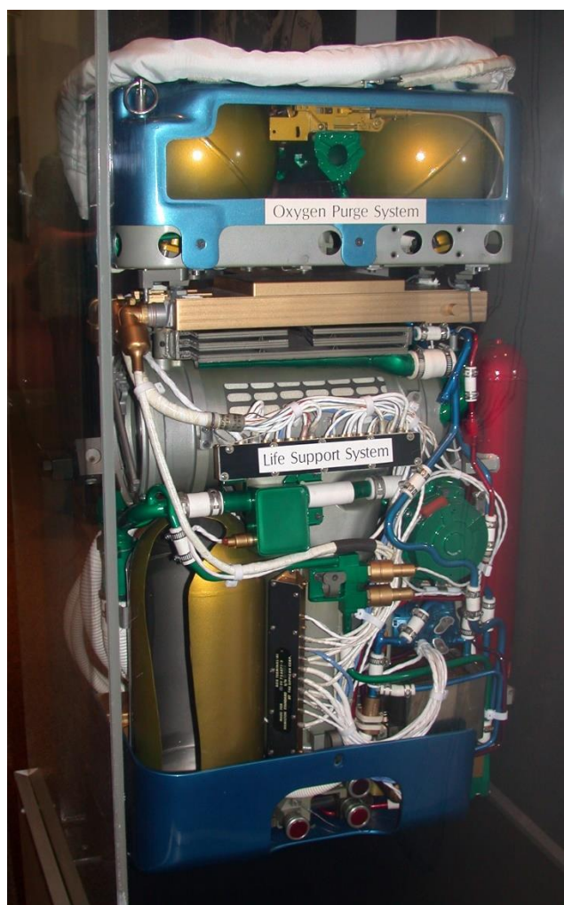
Figure 5. Internals of the Life Support Backpack 8
