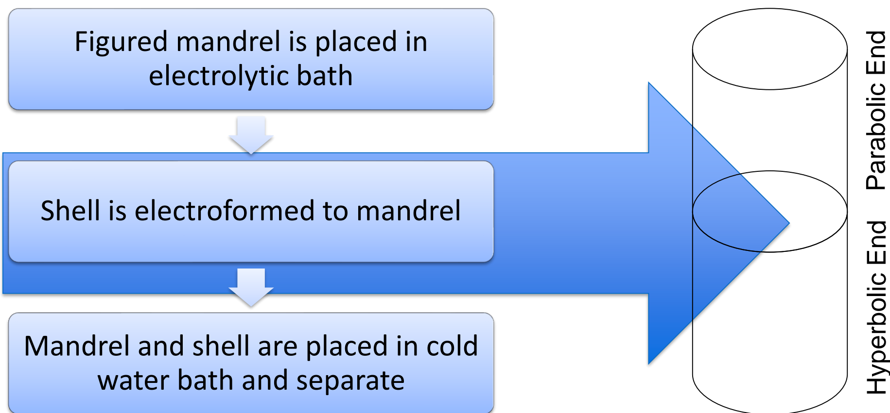
Figure 2: X-ray mirror shell fabrication process
