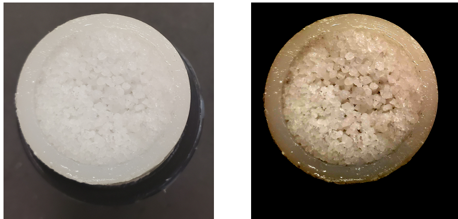
Figure 3.2: 100 micron NPS Specimen Original (left) and Enhanced Contrast to Emphasize Pore Visibility (right) Images
