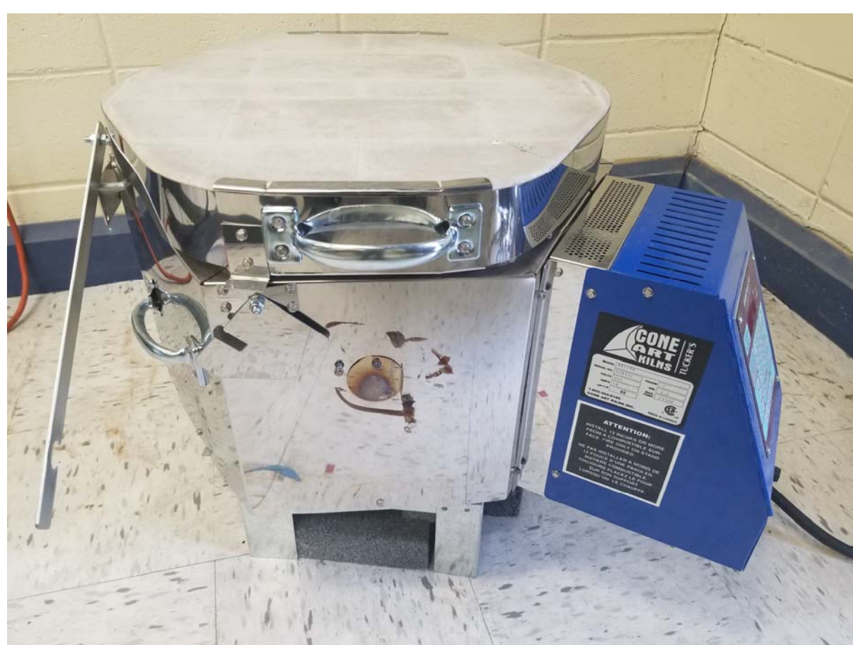
Figure 3- Ceramic pieces were fired in a Cone Art BX119D kiln at cone 8 (about 1250° C)
