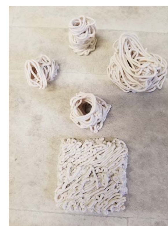
Figure 4- Porcelain pieces were crafted using a syringe to simulate how the paste would behave when driven by a small piston.
