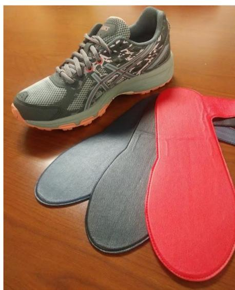
Figure 1 (left): Novel loadsol® sensor compartments. Figure 2 (right): ASICS GEL-Venture 6 running shoes and loadsol® sensors.
