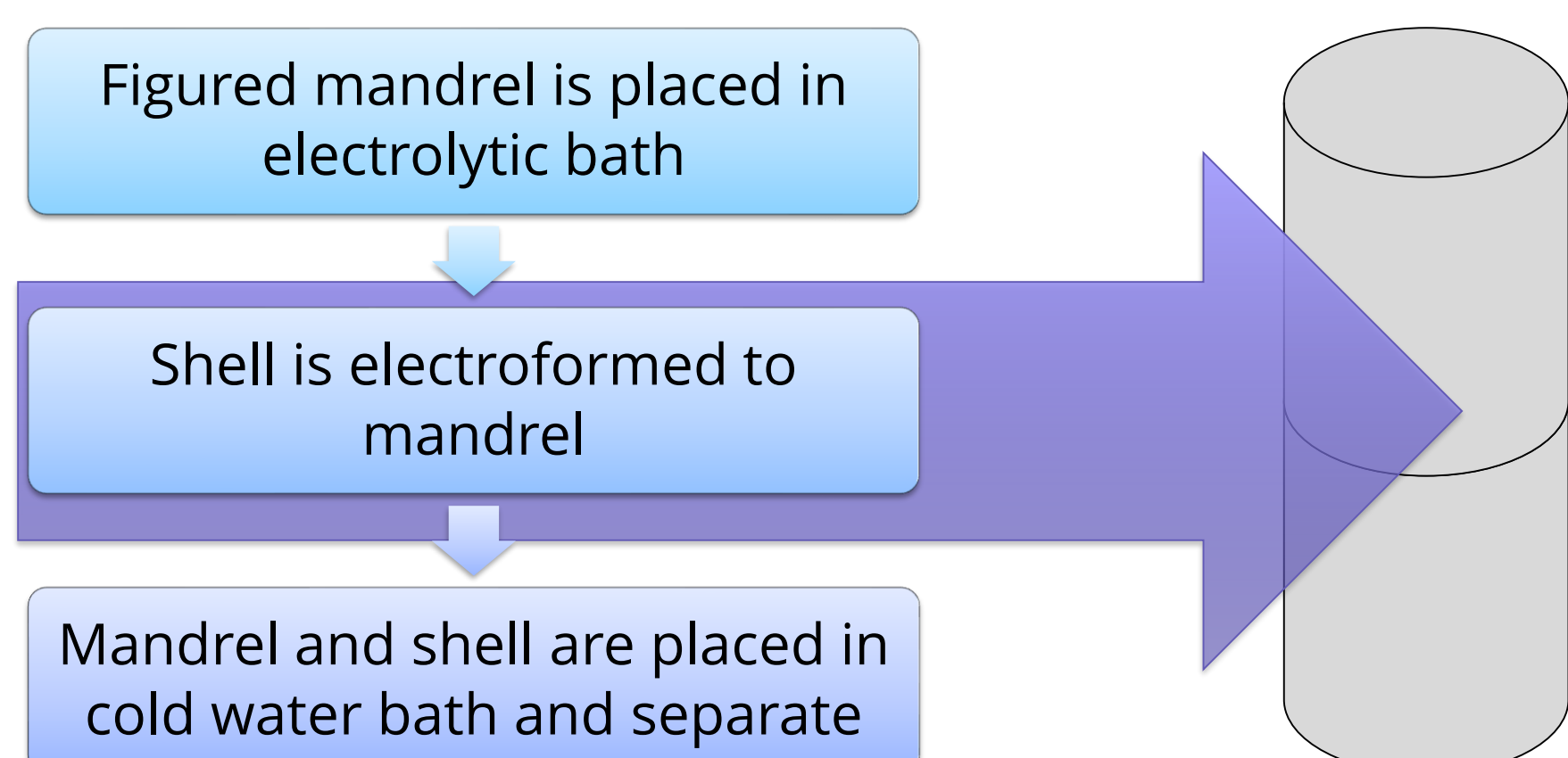
Figure 3: X-ray mirror shell fabrication process
