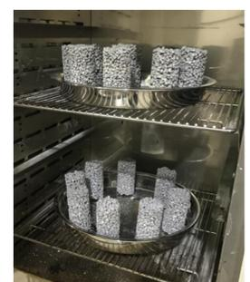
Pervious Concrete samples oven drying
