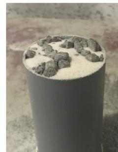
Pervious concrete sample filled with fine silica sand
