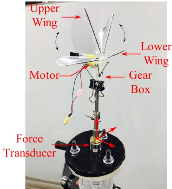
Figure 4: Experimental apparatus. Flapper is mounted on the force measurement test stand.
