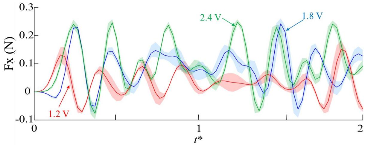
**Figure 9: Time history of force production in the x-direction for two flapping periods.**
