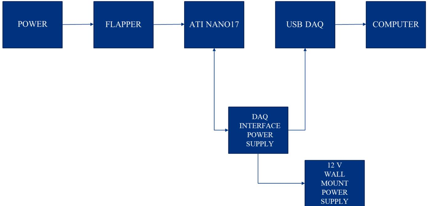
**Figure 5: Experimental method flow chart.**
