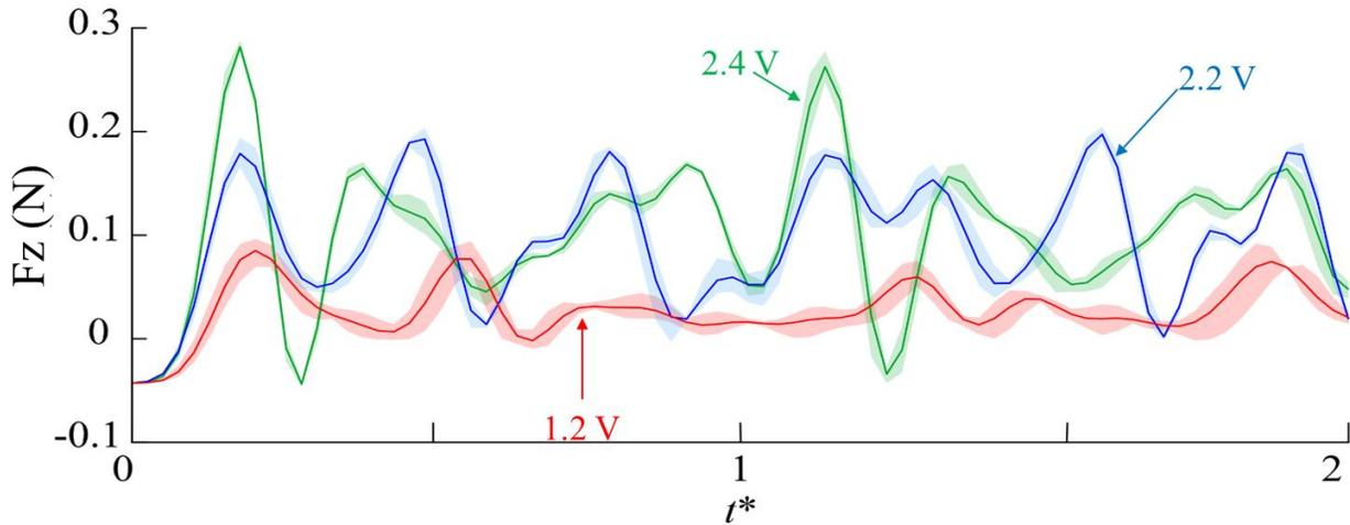
**Figure 8: Time history of force production in z-direction for two flapping periods.**
