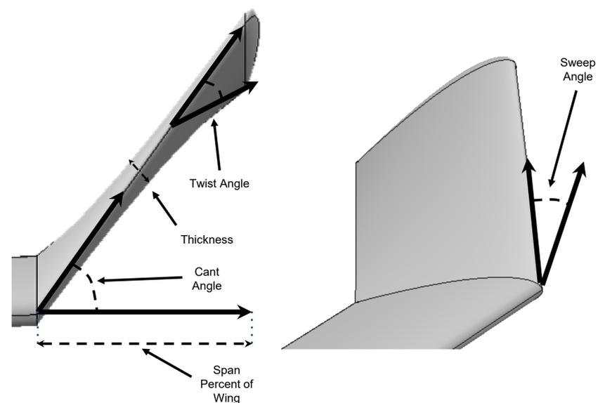
Fig. 1 — Geometrical parameters that define a winglet in the small scale UAV 3D model.
