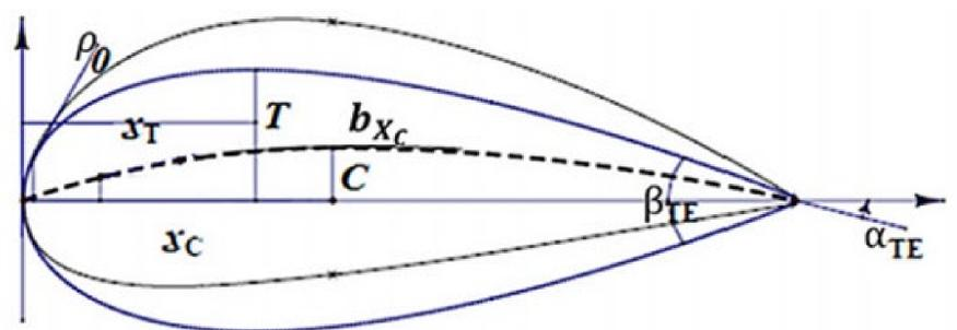
Fig. 2 — Geometrical parameters from the IGP method of parameterizing an airfoil as defined in [1].
