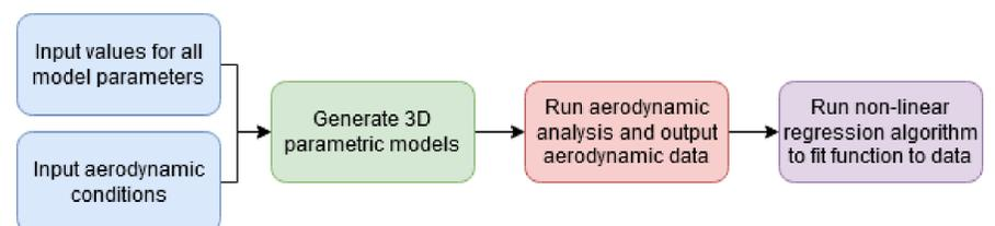
Fig. 3 — Flow diagram for the developed algorithm.
