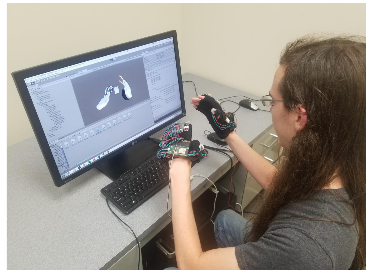
Testing an earlier build of the program. The Unity workstation used to create the program is visible onscreen. The Leap Motion camera is obscured under the left arm.
