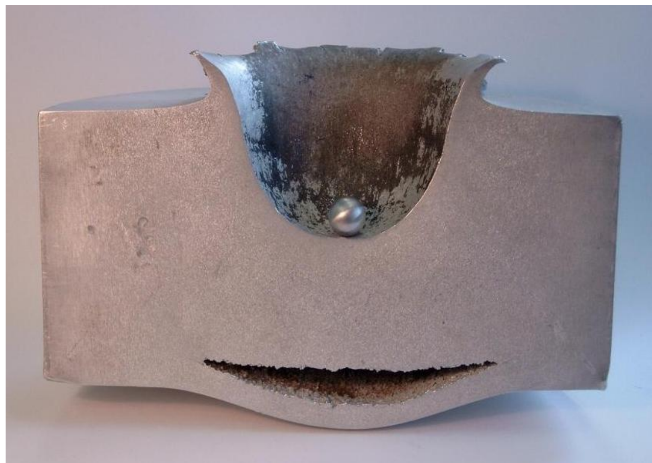
Results of a European Space Agency (ESA) lab test showing results of an impact at 6 km/s between a 1.2 cm aluminum sphere and a 18 cm aluminum block.
