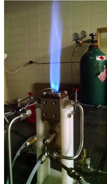
Figure 1. Pentad rocket injector with a methane-air flame on the lab bench.
