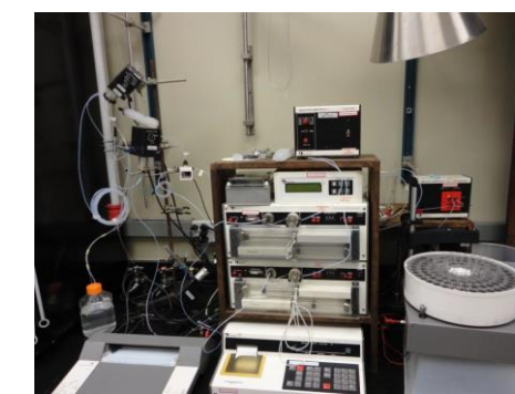
Figure : Nickel column (FPLC) apparatus
