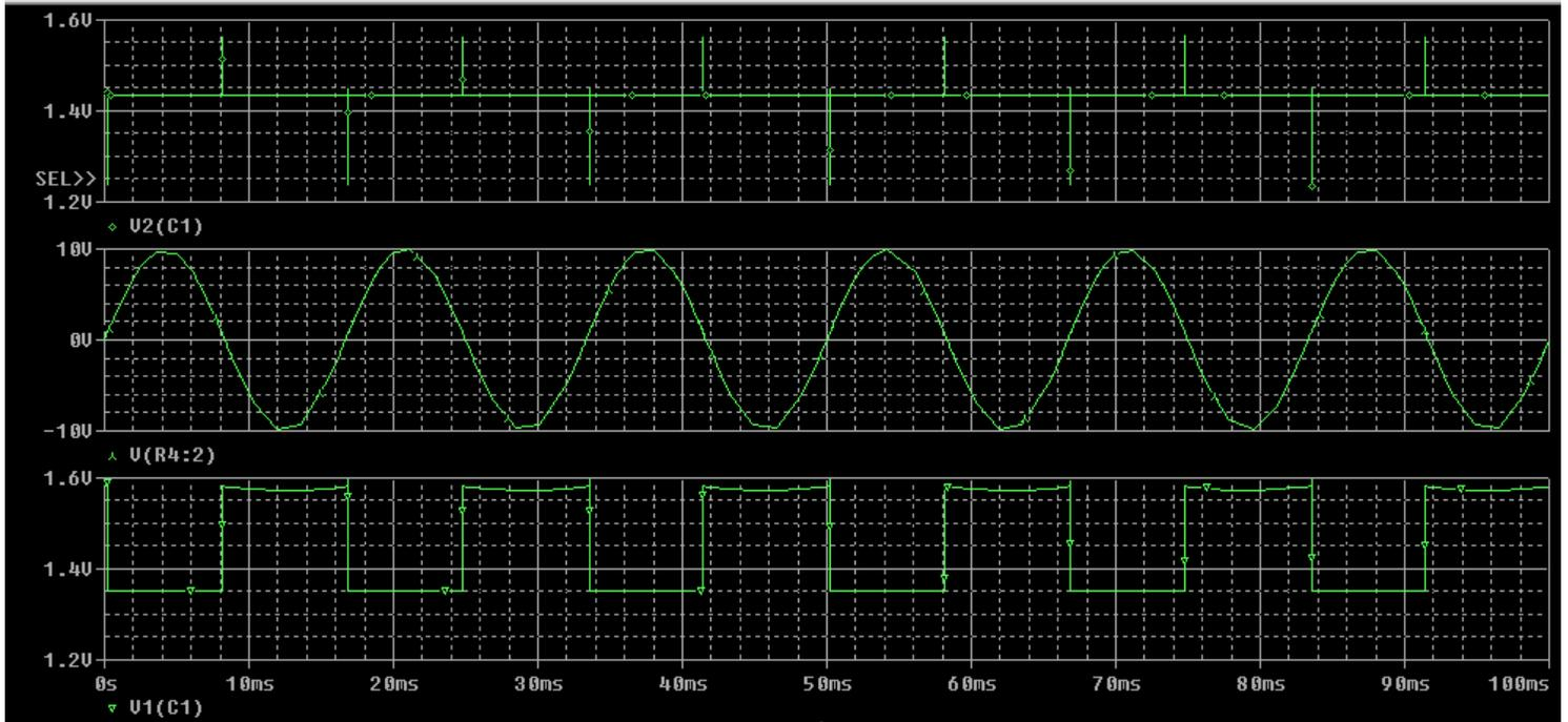
The figure above shows the PSPICE simulation of the voltage across capacitor C1 as a function of time under ideal conditions. The figure below is the same simulation, but capacitor C1 has been replaced with another capacitor with 1000 times more capacitive ability. This particular switch was performed because the numbering system on capacitors is incredibly small, and accidentally installing a capacitor with 1000 times the storage capability is a completely plausible construction error.
