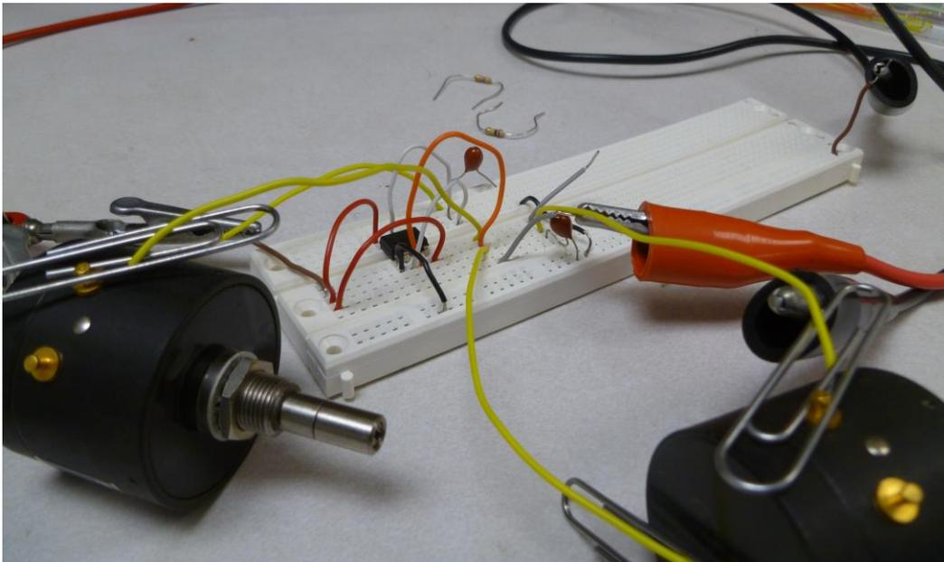
555 Astable Multivibrator with component potentiometers
