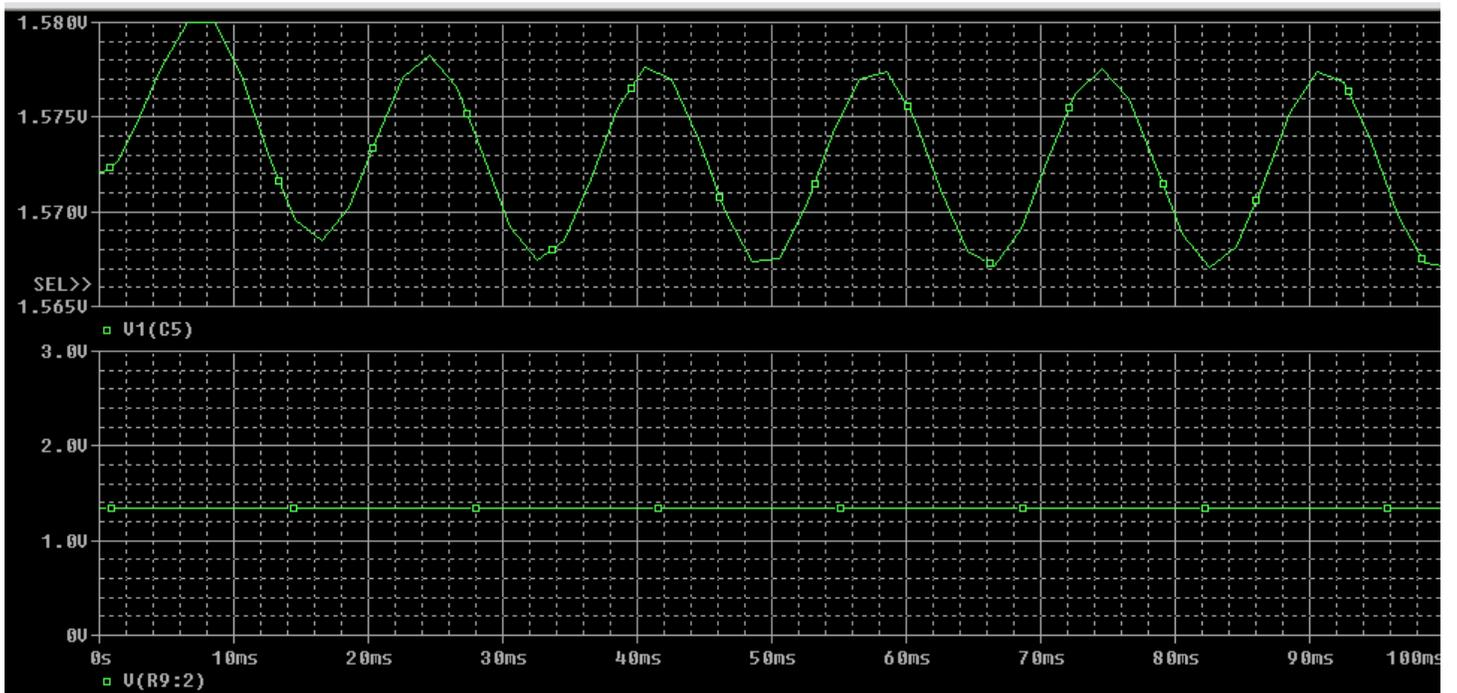
The figure above is the output from the LM353 when the resistor grounding the op-amp is increased by a factor of one million.
