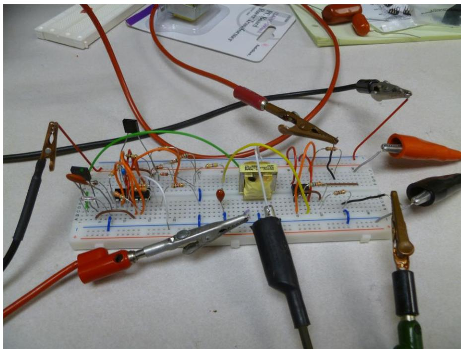
SID Receiver Undergoing Testing / Calibration
