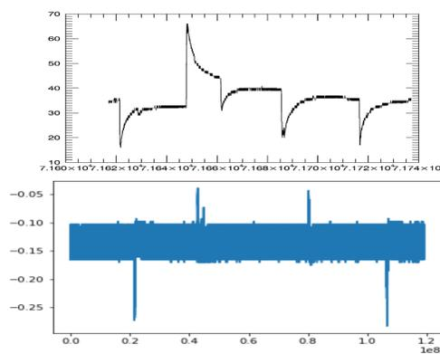
*Left: Above is data from the electric field mill at SWIRLL showing the Voltage over 2 minutes; below is the same 2 minutes of data and the Voltages picked up by the Arduino EFM project. Sample is taken from 19:53:37-19:55:37 on 8/4/2017.*
