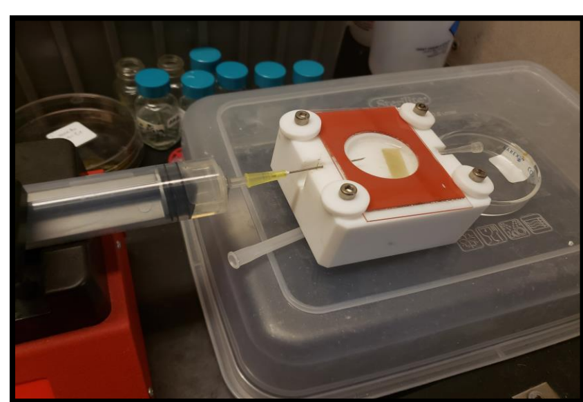
Fig 2. Flow Chamber containing Gold Nanostructures on a Glass Slide
