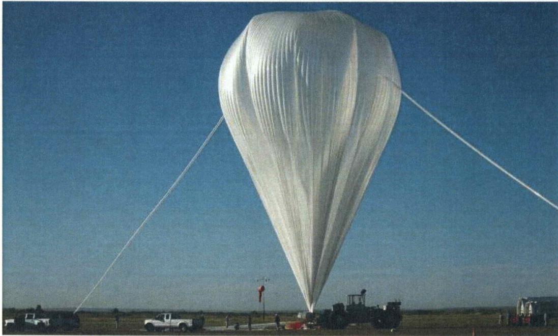
Figure 2.3: Image of a zero pressure balloon right before launch. Image credit: NASA/MSFC. [26]
