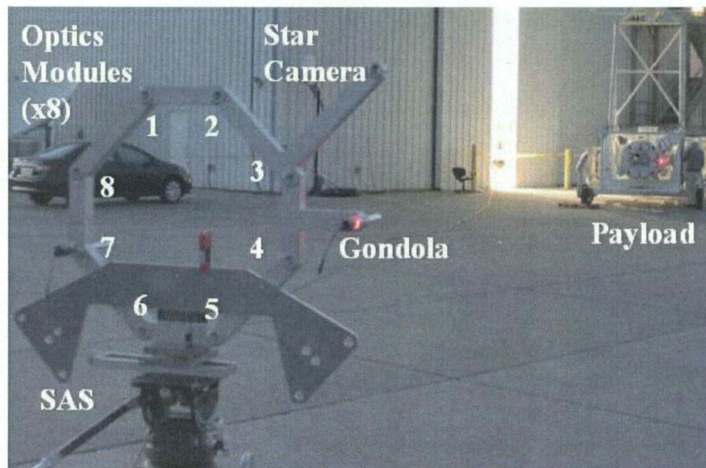
Figure 2.8: Alignment fixture used to align the optics modules of the HEROES payload. Image credit: reproduced with permission of IEEE. © [2014] IEEE. [29]
