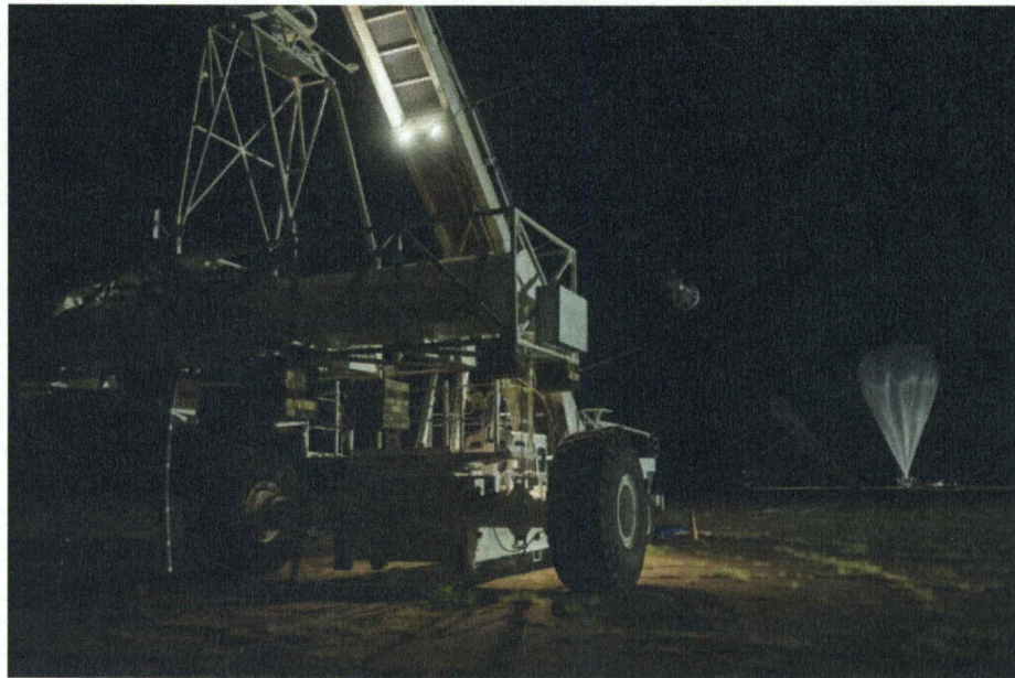
Figure 5.1: HEROES payload right before launch. The balloon is inflated in the background with the payload attached to the flight train and launch vehicle. Image credit: reproduced with permission of IEEE. © [2014] IEEE. [29]
