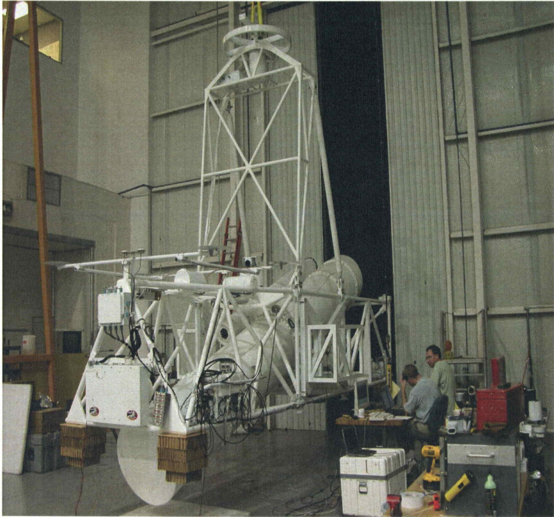
Figure 4.9: Image of the HEROES payload elevated off the ground using a crane for a hang test at Fort Sumner, N.M. Image credit: NASA/MSFC.
