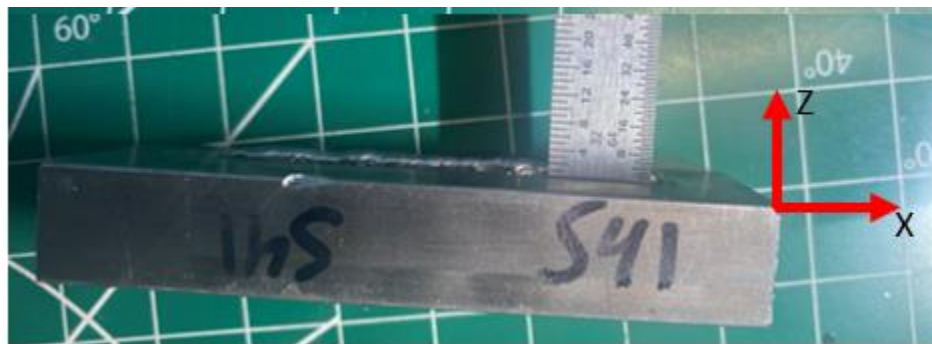
Figure 4.2: Single Layer Representative Deposition and Coordinate System of Sub-sample Face (Side View) – XZ Intersection Represents the Origin.
