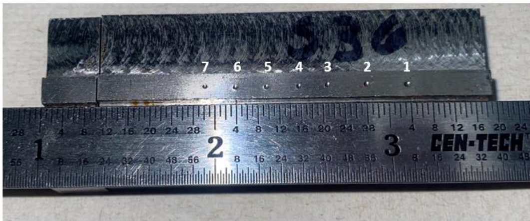
Figure 4.19: Hardness Validation Measurement Locations Along the plan view of the Machined Width (Plan View).
