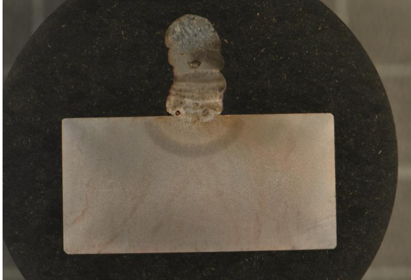
Figure 4.32: Representative Polished and Etched Sample of Sub-sample Face – S45 Ten-Layer Heat-Treated Sample with Waterless Kallings Etchant.
