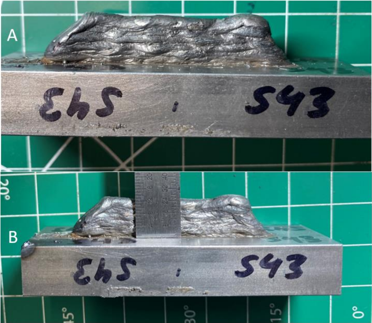
Figure 4.11: Ten-layer Nominal (A) and Heat-treated As-Built (B).
