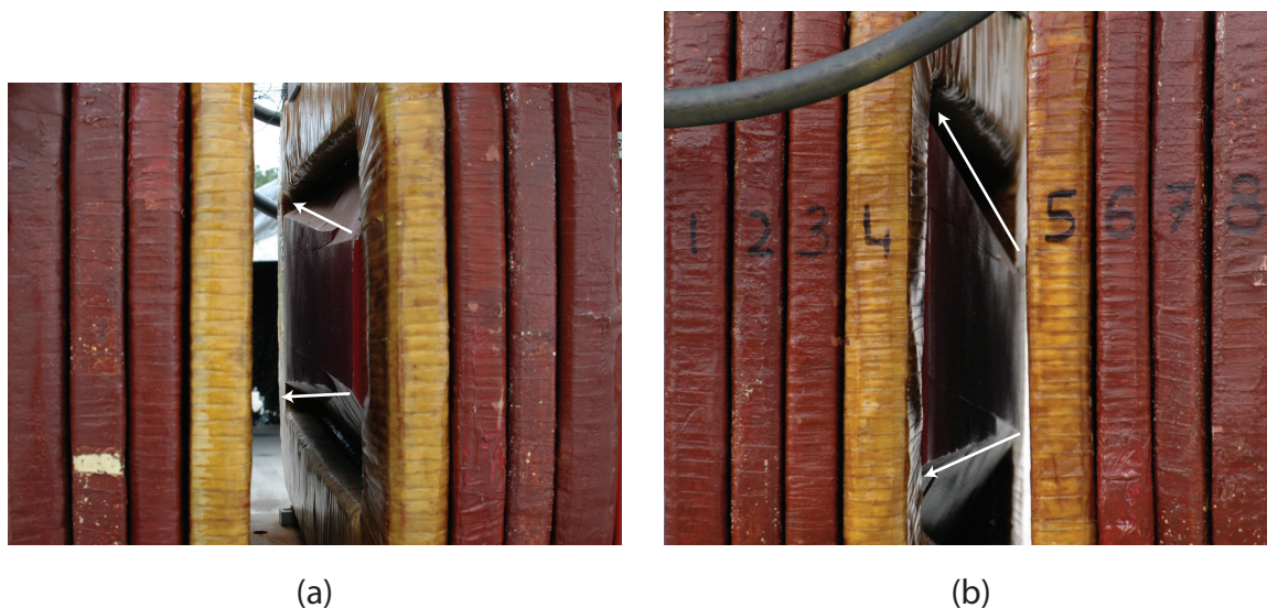
Figure 5.10: Close-up photographs of the MAPX electromagnet, showing the increasing surface area of the magnetic poles, which effectively lowers the intensity of the magnetic field in the downstream region of the MAPX channel. Part (a) is the view of the poles from the upstream end of the magnet, while (b) is the downstream view. The white lines/arrows show the poles divergence in each photo.
