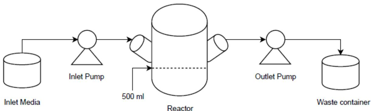
Fig 1. Diagram of the Bioreactor system.
