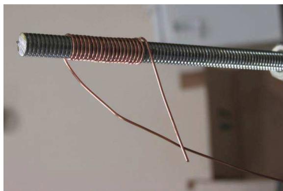
**Figure 3.** Coil antenna fabrication.
