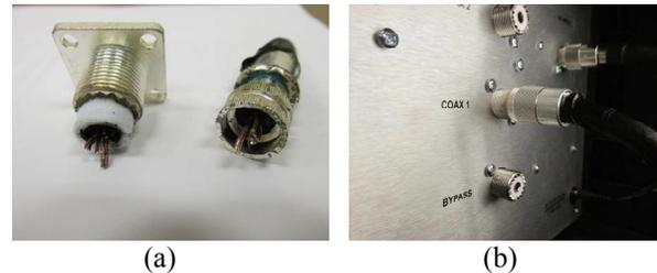
**Figure 10.** (a) Coaxial cable connector after power sent to a connection. (b) Coaxial cable re-soldered to the matching network after RF transmission.
