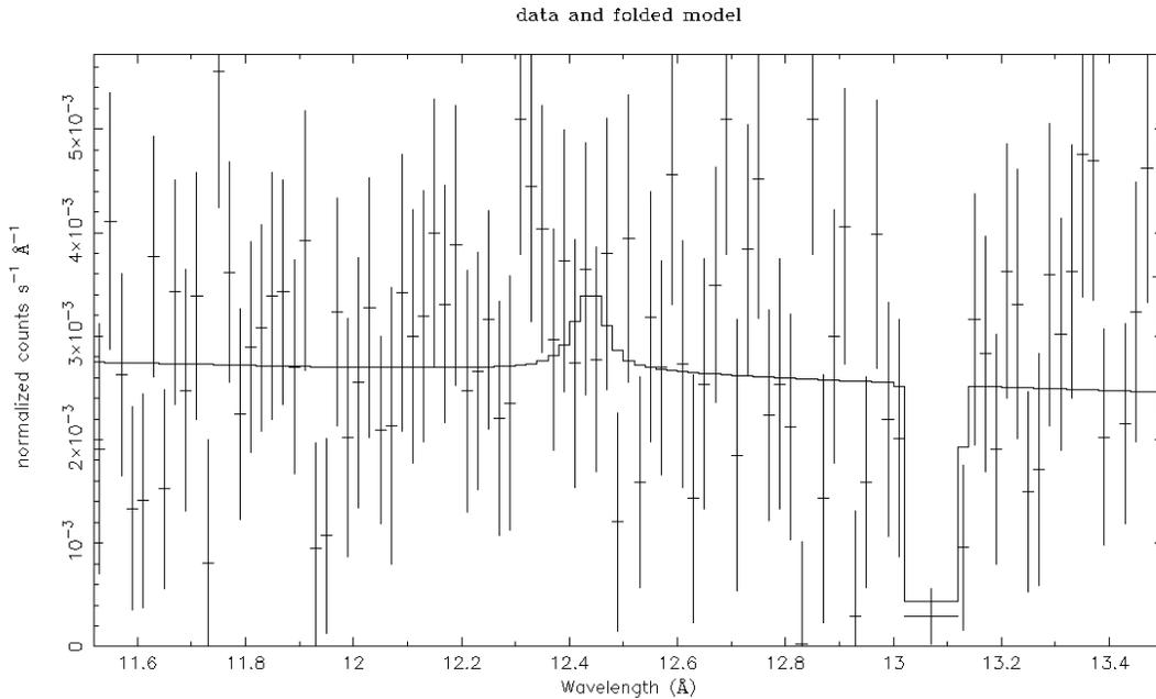
Fig. 4 – The NeIX data does show some evidence of an absorption line, but is unfortunately of  $<2\sigma$  significance. The area around Ne IX contained several instrument artifacts that required the parsing out of some data.
