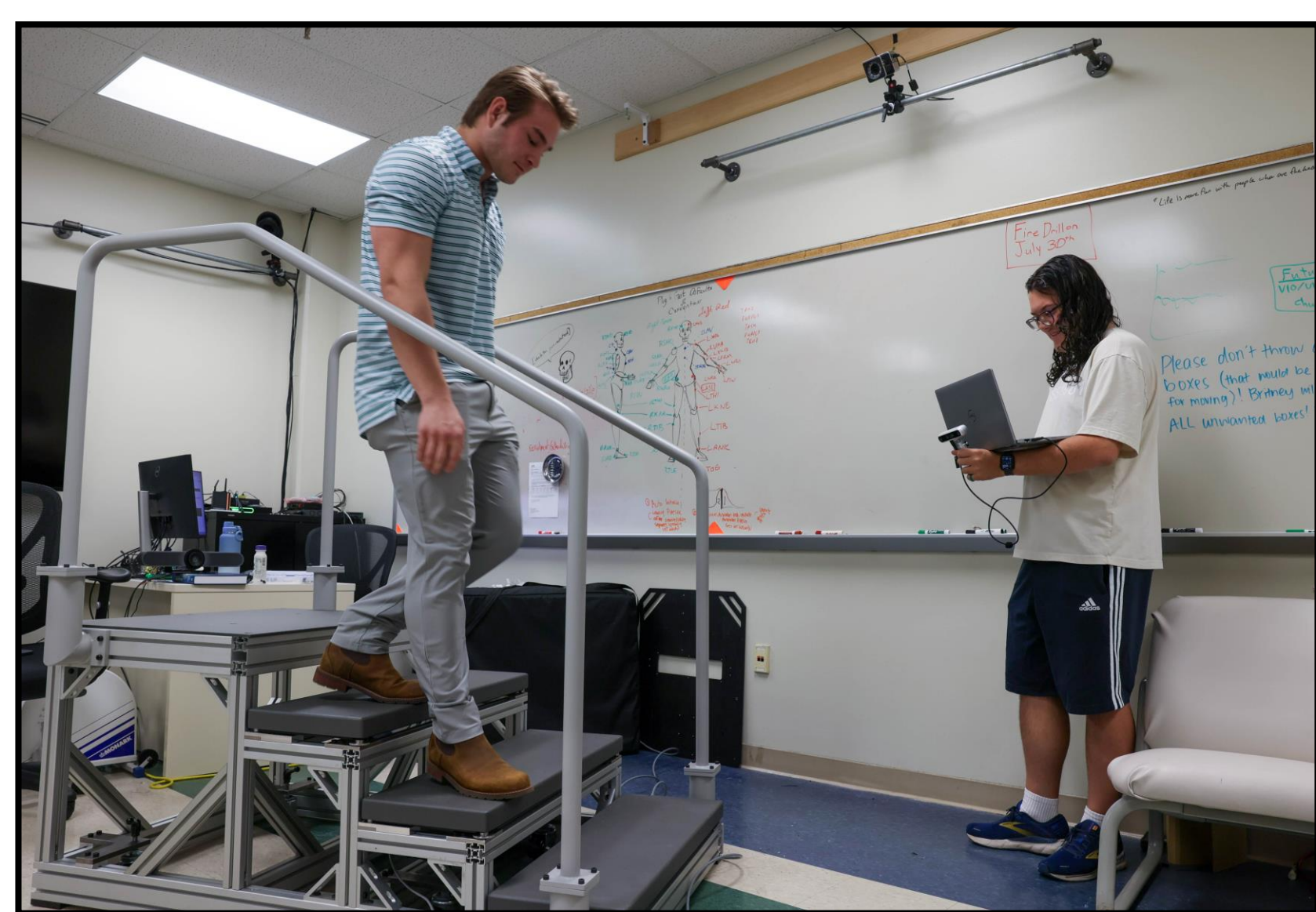
Figure 4. Lab instrumented stairway
