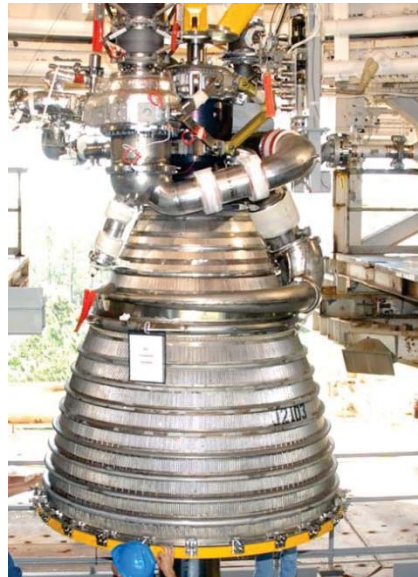
Figure 1.2 J2-X engine, to be used on the upper stage of the Space Launch System [5].
