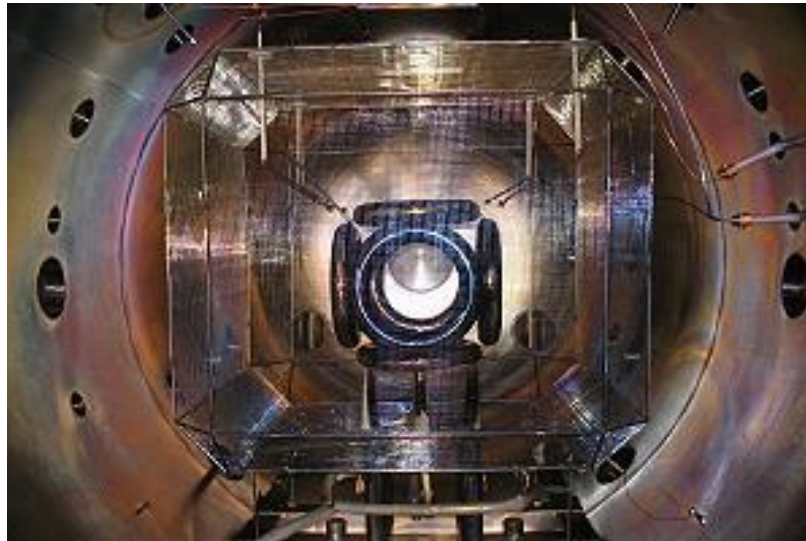
Figure 1.1: Inertial Electrostatic Fusion (IEF) device being developed at EMC2 [49].
