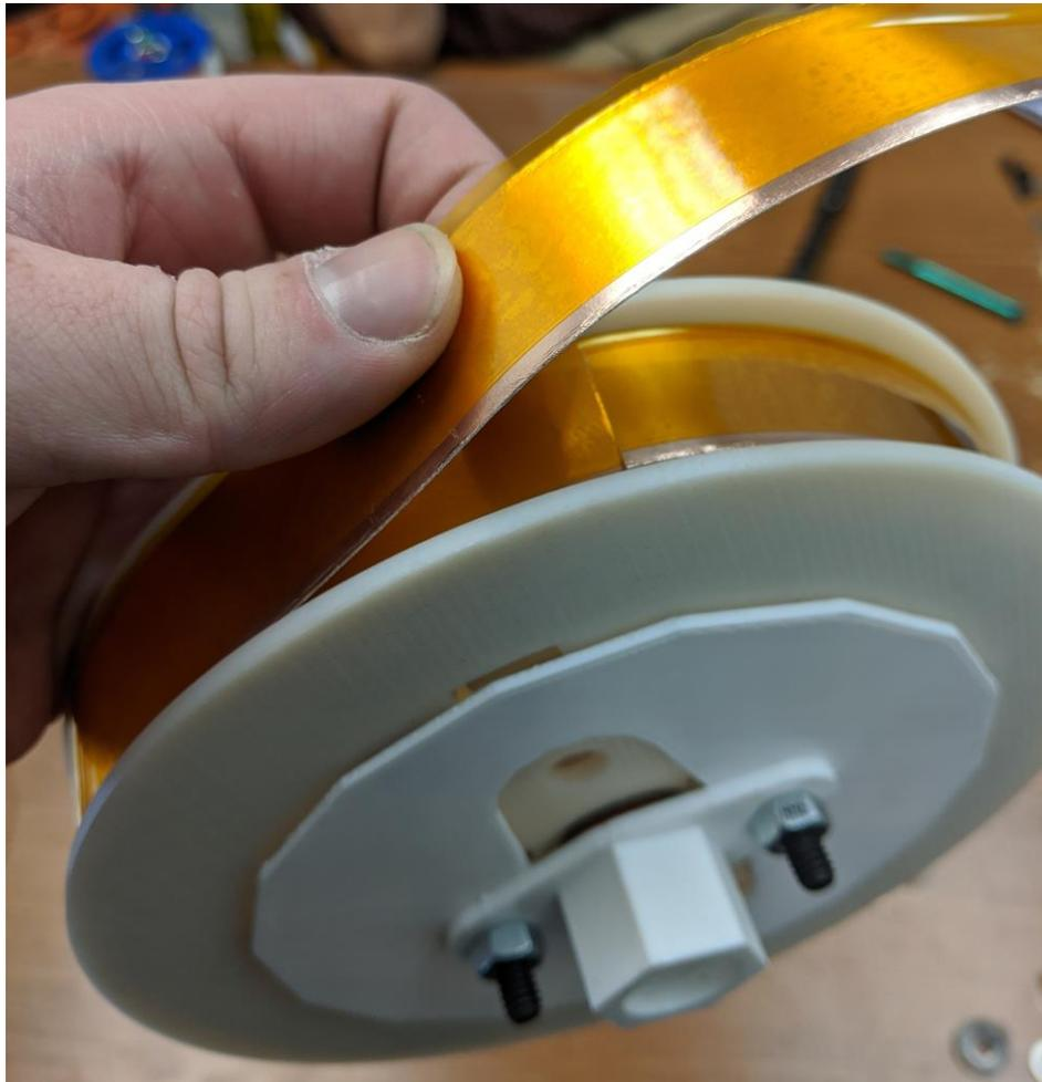
**Figure 3.14** A 30-turn spiral generator fabricated as a first test.
