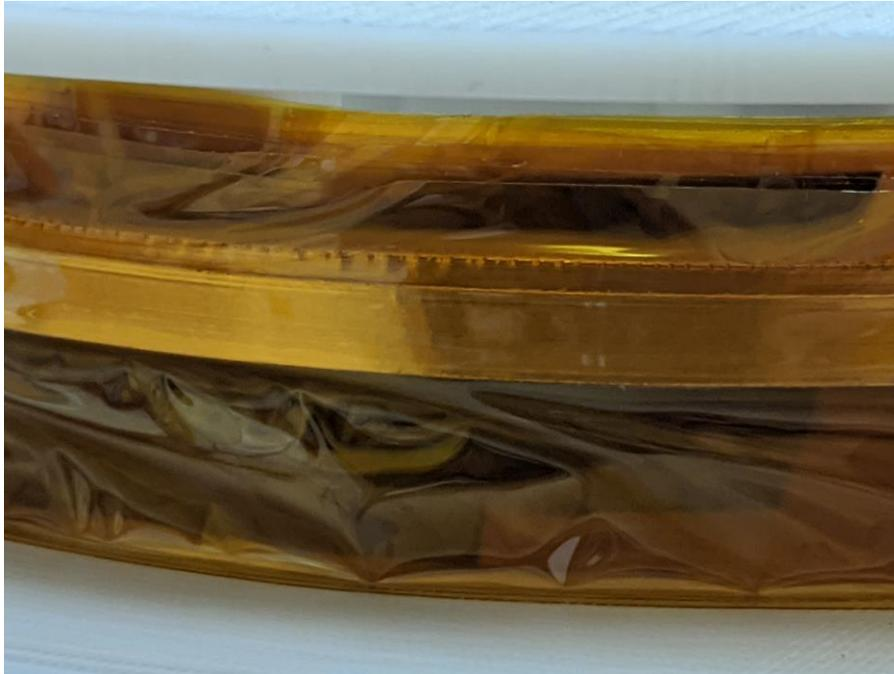
**Figure 3.16** A close up view of the 52-turn spiral generator.
