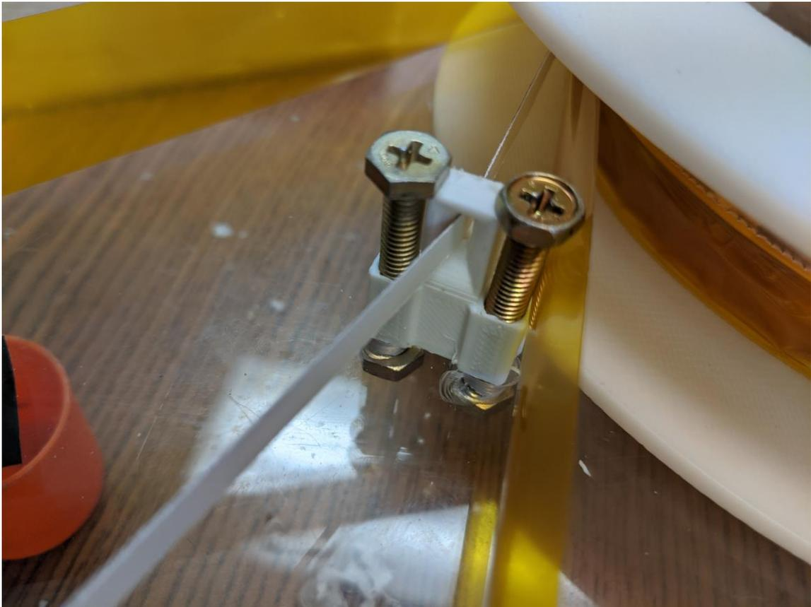
**Figure 3.12** Alignment and Friction Gate used for Winding in Progress.
