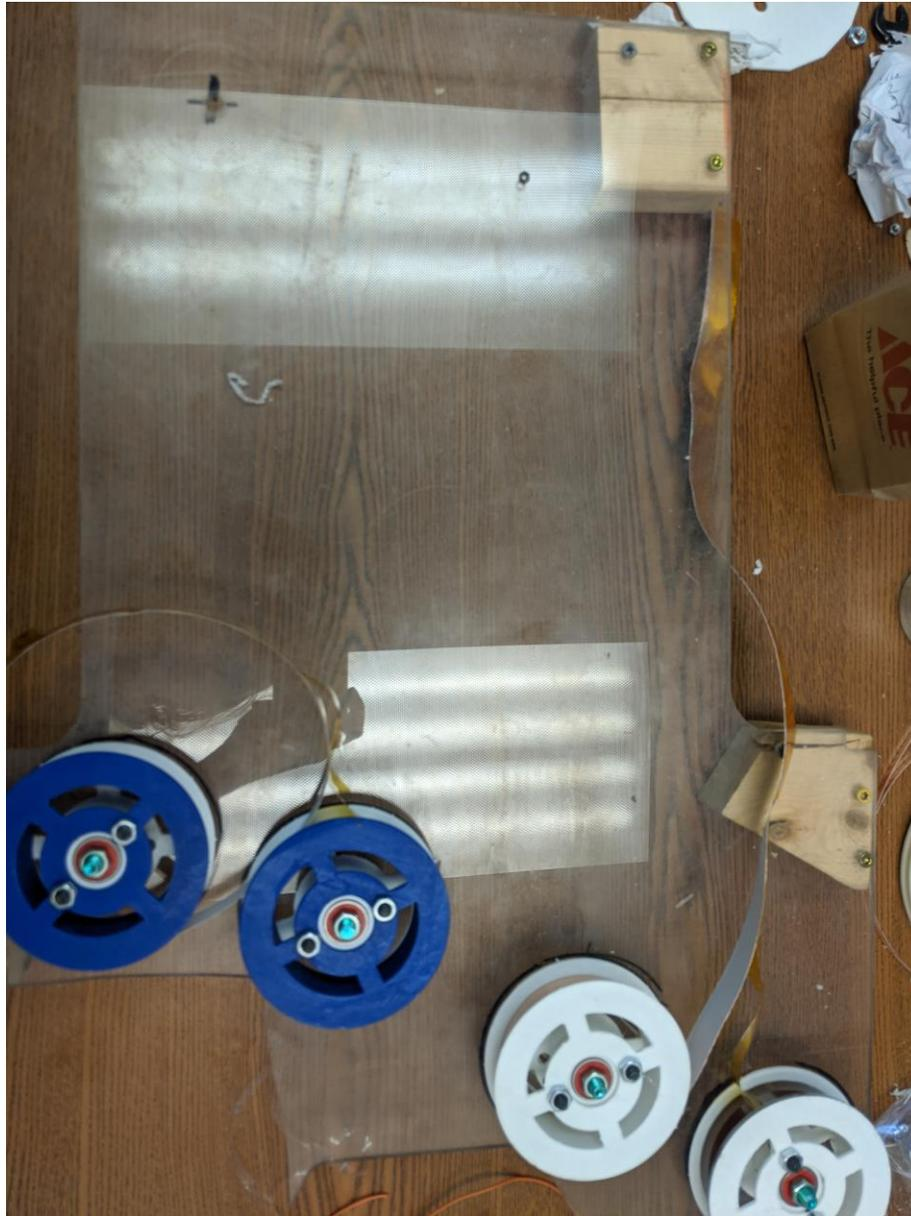
**Figure 3.11** Winding System Used for Fabrication.
