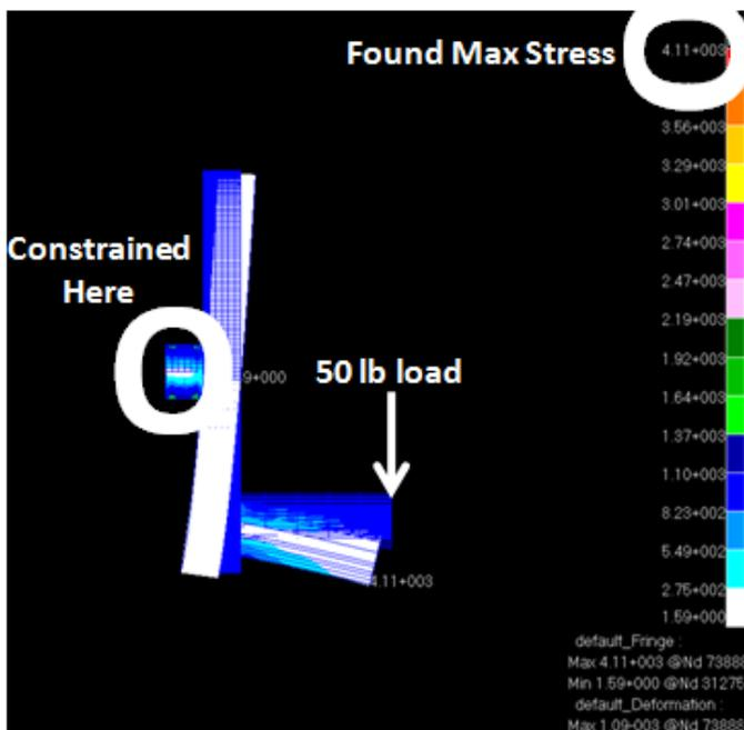
Figure 4. Results of Finite Element Analysis of Crank Shaft Handle (side view)
