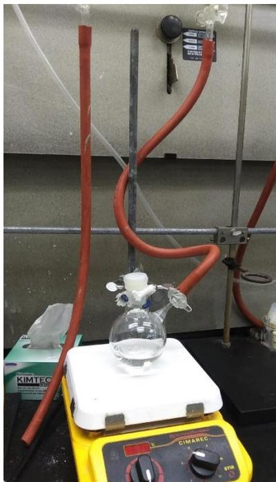
**Figure 2:** Sealed Schlenk flask attached to the Schlenk line.<sup>[8]</sup>
