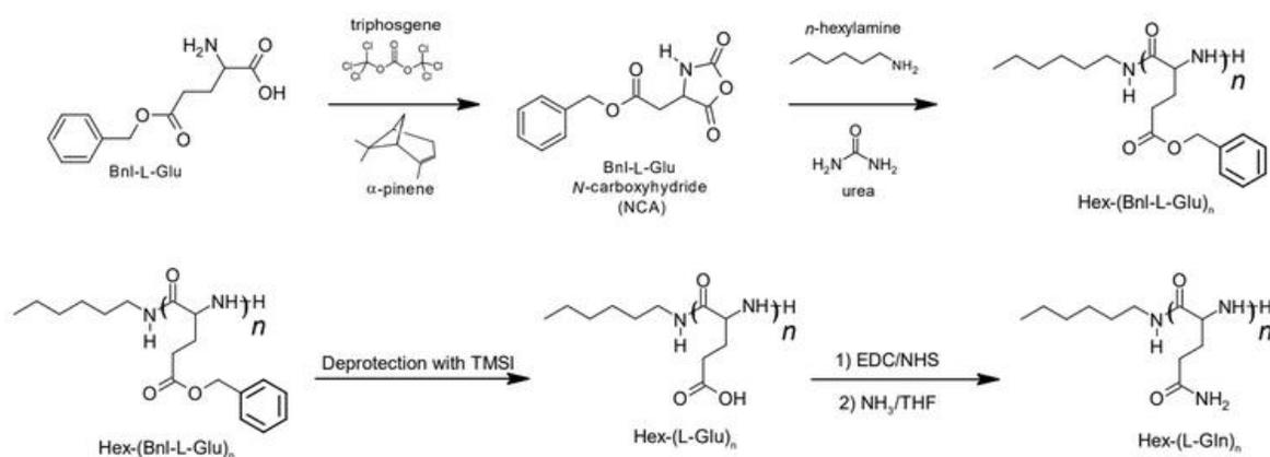
**Figure 1:** Reaction scheme for the synthesis of hex-poly(glutamine).<sup>[6]</sup>
