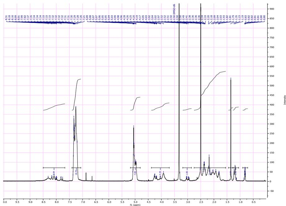
**Figure 5:** NMR spectrum of the 20-length hex-poly(benzyl-L-glutamic acid) in DMSO.
