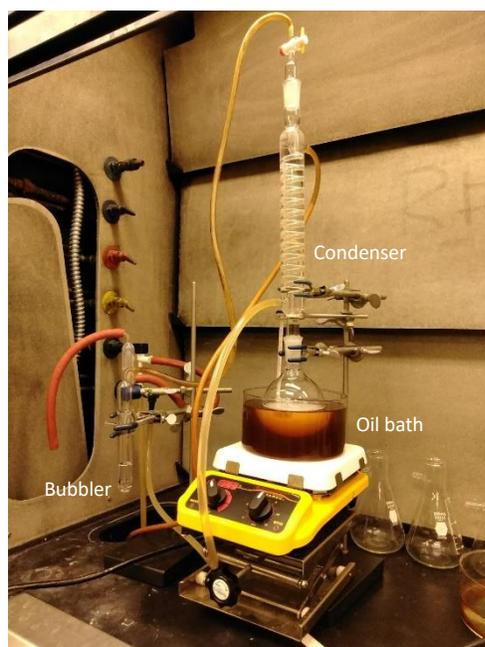
**Figure 1:** Apparatus for the synthesis of NCA.<sup>[7]</sup>
