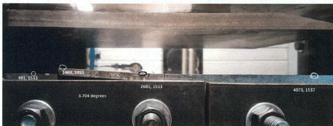
Figure 3.32: An example image showing the choking flap angle calculation.
