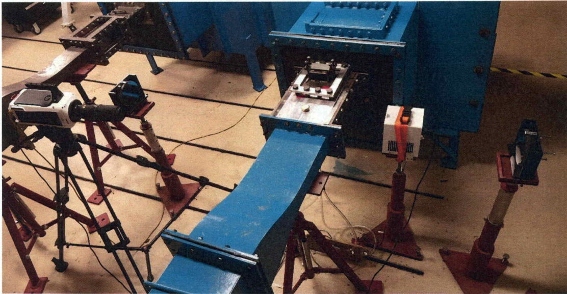
Figure 4.5: Photograph of the flow visualization system.
