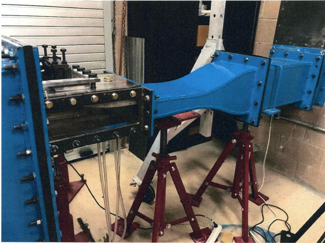
Figure 3.31: The nozzle and test section.
