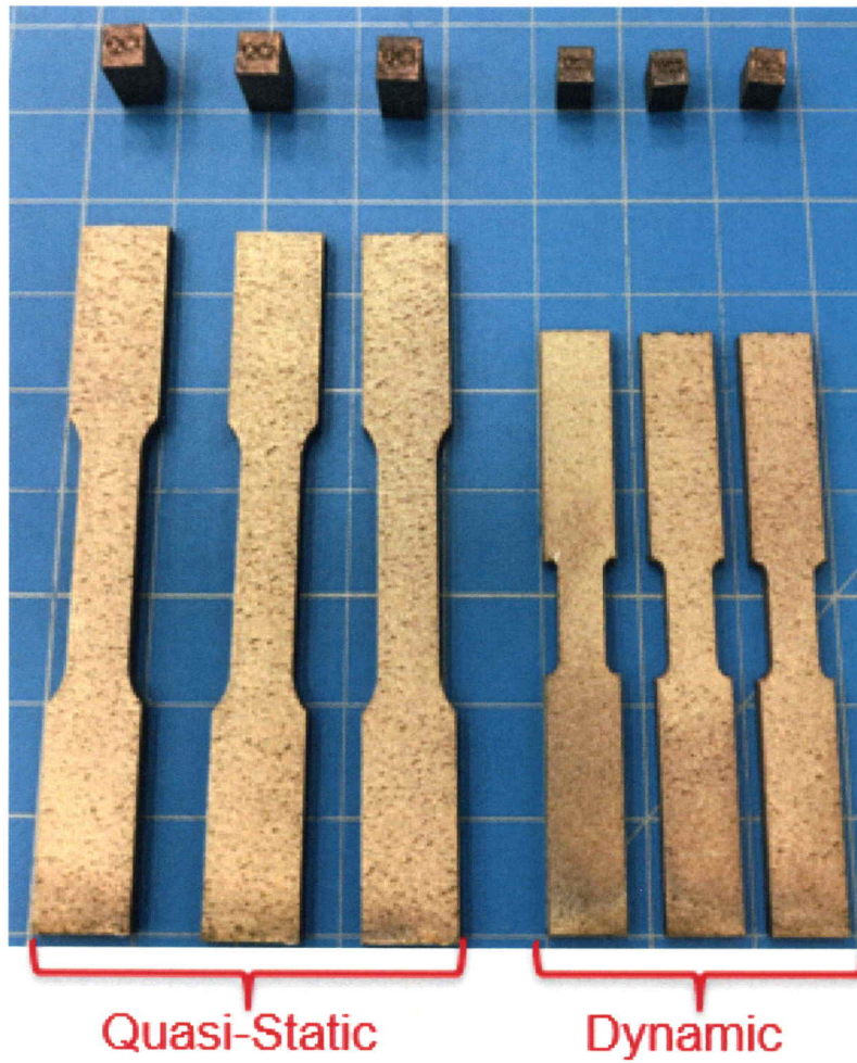
Figure 3.3: The AM bulk tension and compression samples used for quasi static (left) and dynamic (right) testing
