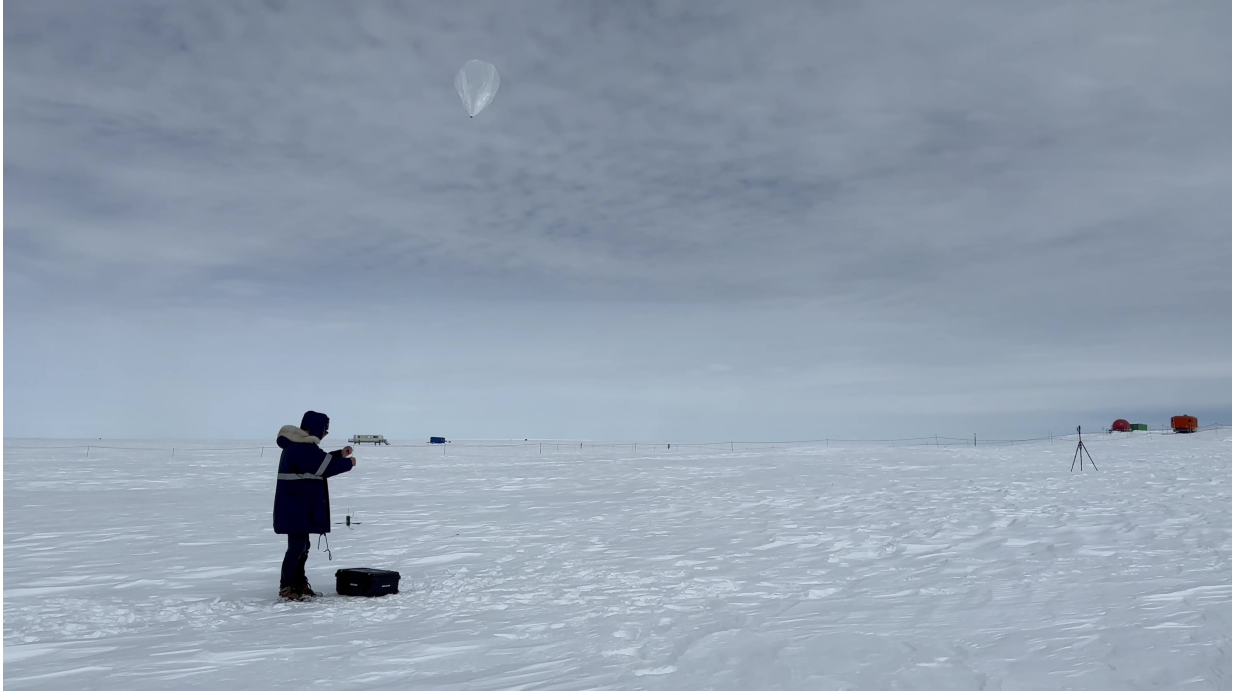
Figure 1.1: Micro super pressure balloon tethered shortly before launch. Transmitter is below the hands of the person launching. Neumayer station is in the background.
