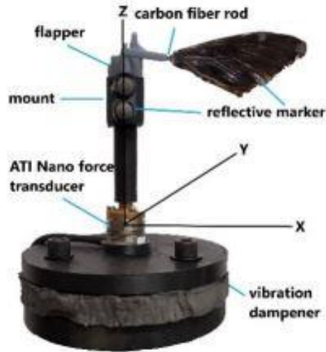
Figure 3.4 Flapping wing mount showing the in-house designed flapping mechanism and vibration dampening base. The wing is attached to the flapper using a circular 1 mm diameter carbon fiber rod. From Morris [34]. Reprinted with permission.
