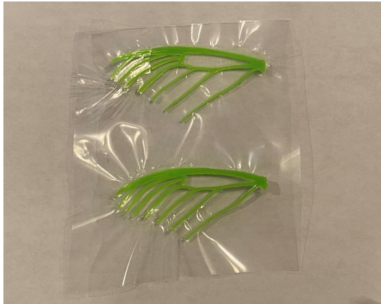
Figure 3.1 Two bonded wings shown after the PLA vein structure (green) has been fused to the PLLA membrane (clear).
