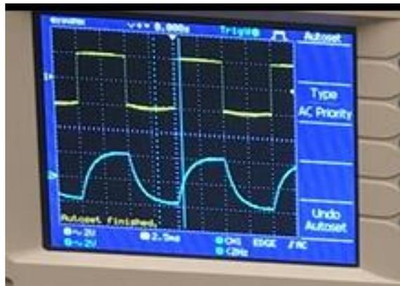
**Figure 5:** Oscilloscope Screenshot of Circuit Square Wave (yellow) and Capacitor Square Wave (blue)
