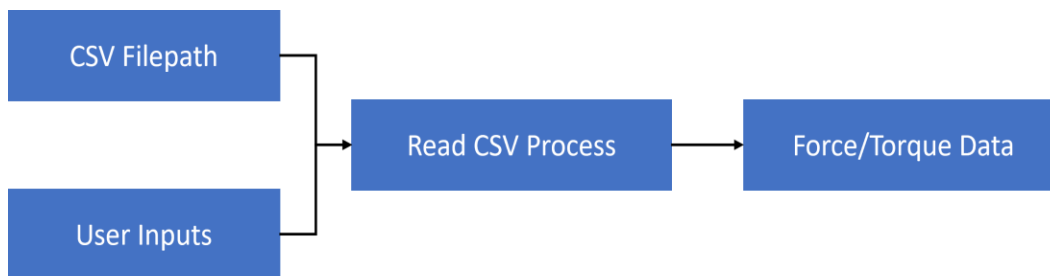
Figure 3.6 Process diagram for the acquire data algorithm. The diagram includes the primary inputs and sequential steps that the algorithm executes to load data previously acquired.
