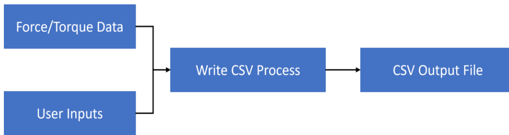
Figure 3.5 Process diagram for the save data algorithm. The diagram includes the primary inputs and sequential steps that the algorithm executes to save acquired data.
