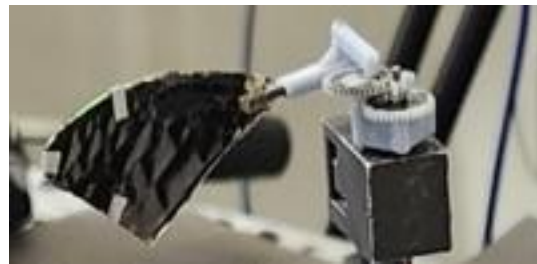
Figure 1.2 Micron wing flapper, with the artificial wing mounted on the left side.
