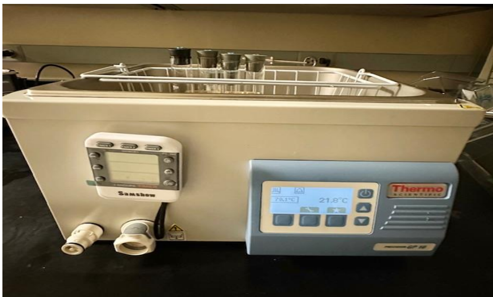
Figure 3.7 Hot bath for glass functionalization. A metal basket was used to hold glass test tubes in place while they are immersed in the hot water bath.
